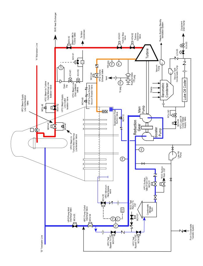
Figure 10.1-1 High Pressure Coolant Injection System
