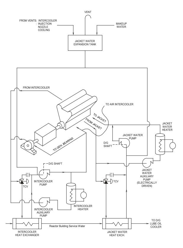
Figure 9.2-5 DG Cooling Water System
