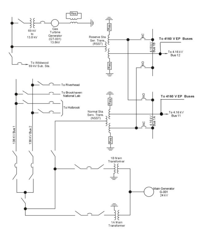
Figure 9.2-1 Main Line Plant Distribution
