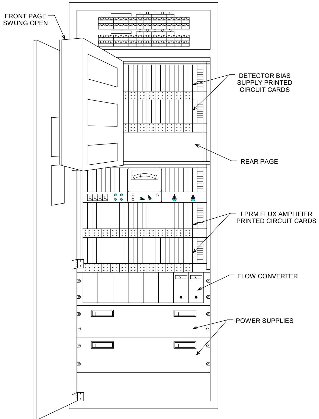
**Figure 5.3-6 Neutron Monitoring Cabinet Layout**
