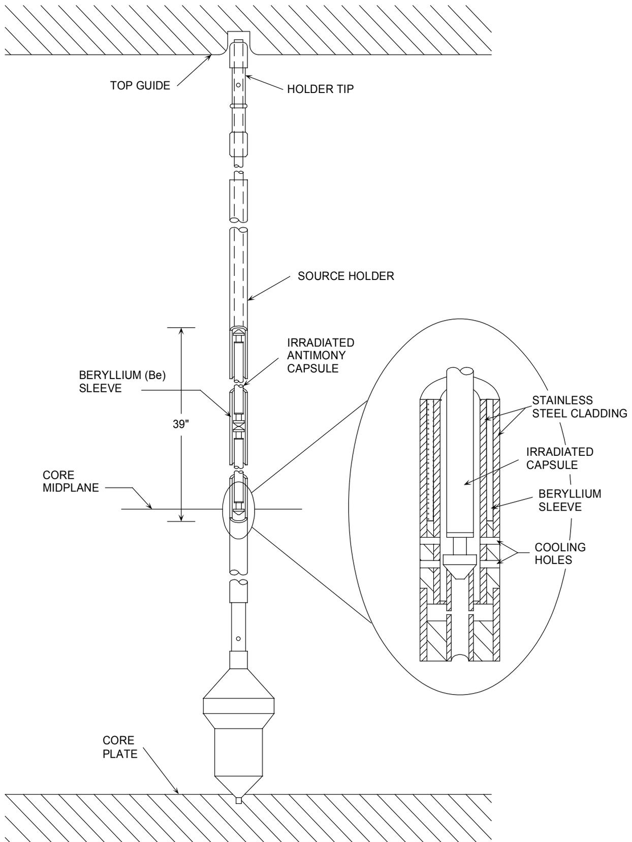
**Figure 5.1-8 Neutron Source Tube**
