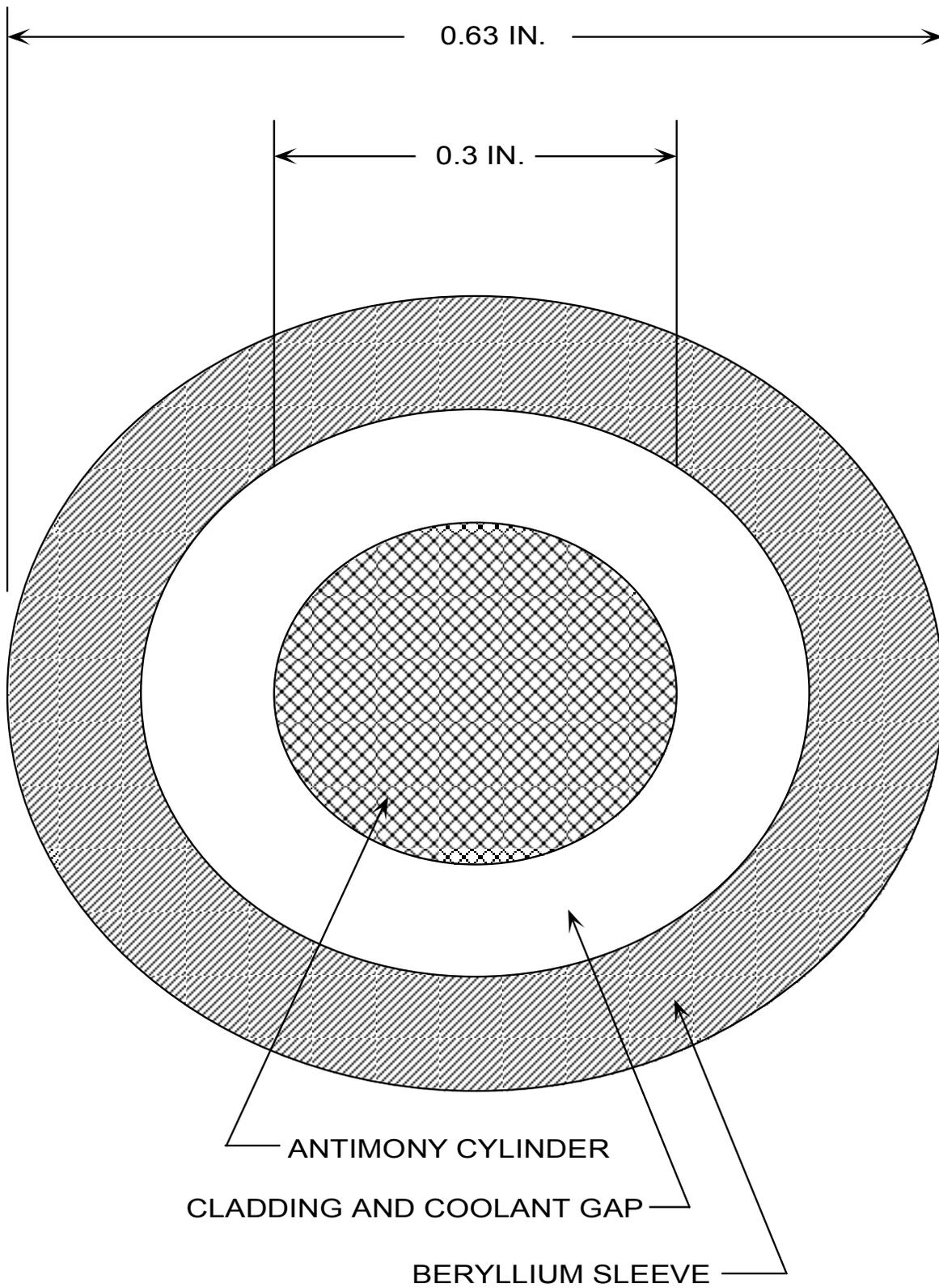
Figure 5.1-9 Neutron Source Configuration
