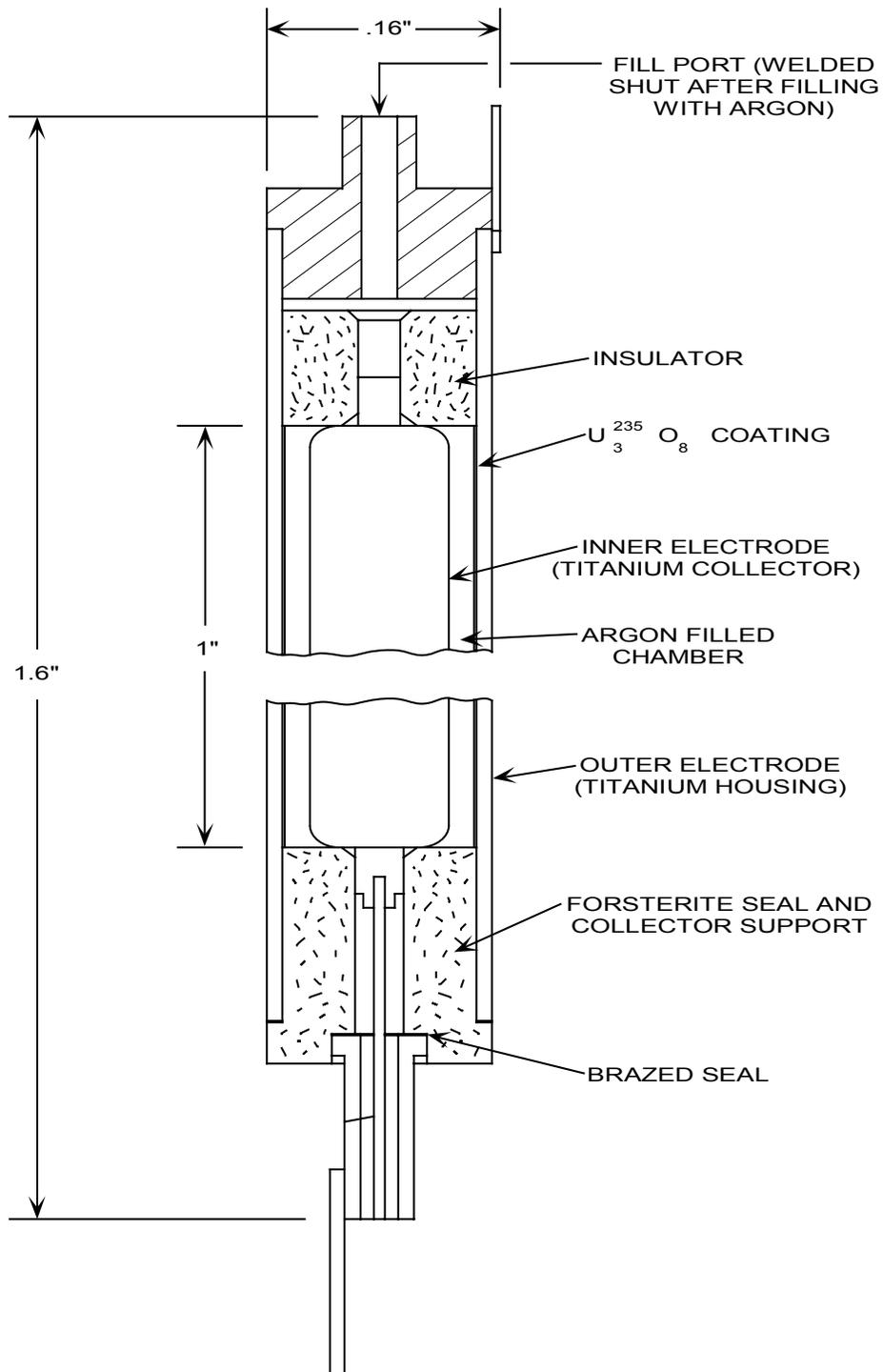
Figure 5.1-2 SRM Fission Chamber
