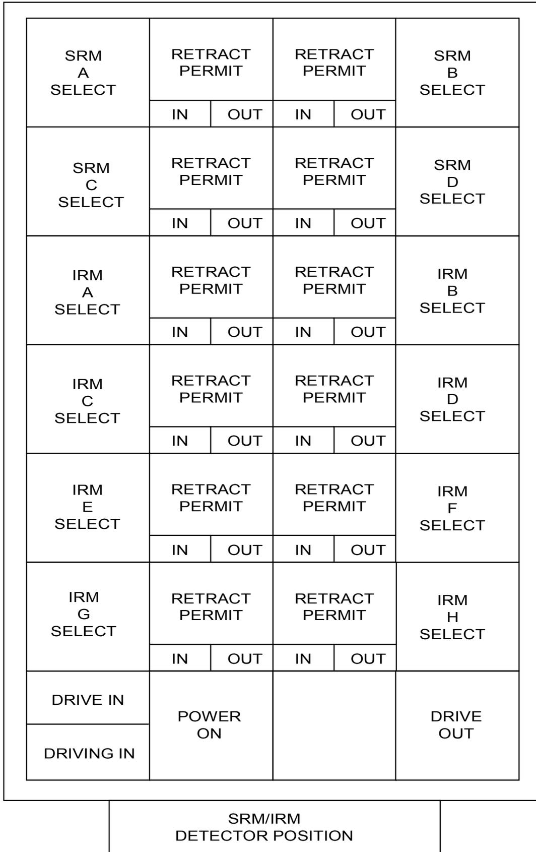
Figure 5.1-6 Detector Drive Control Switch Arrangement
