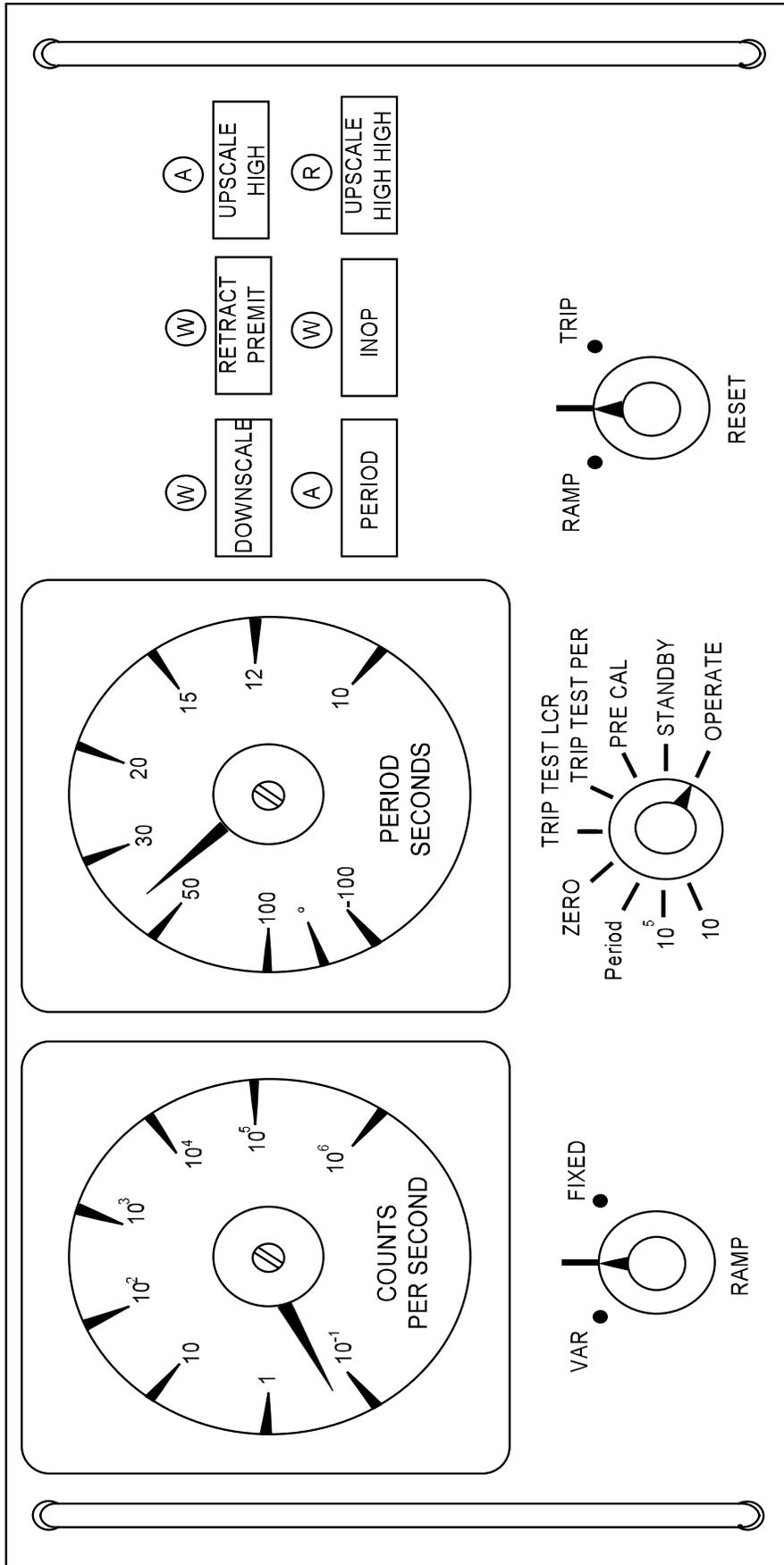
Figure 5.1-7 SRM Drawer Front Panel Layout
