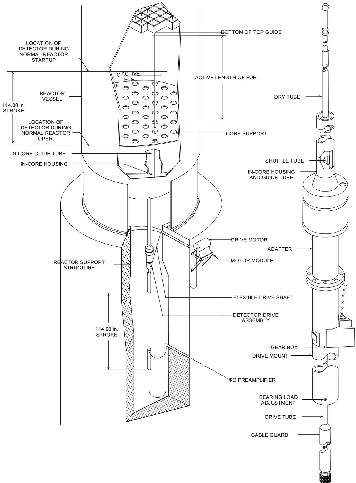
**Figure 5.1-5 Source Range and Intermediate Range Detector**
