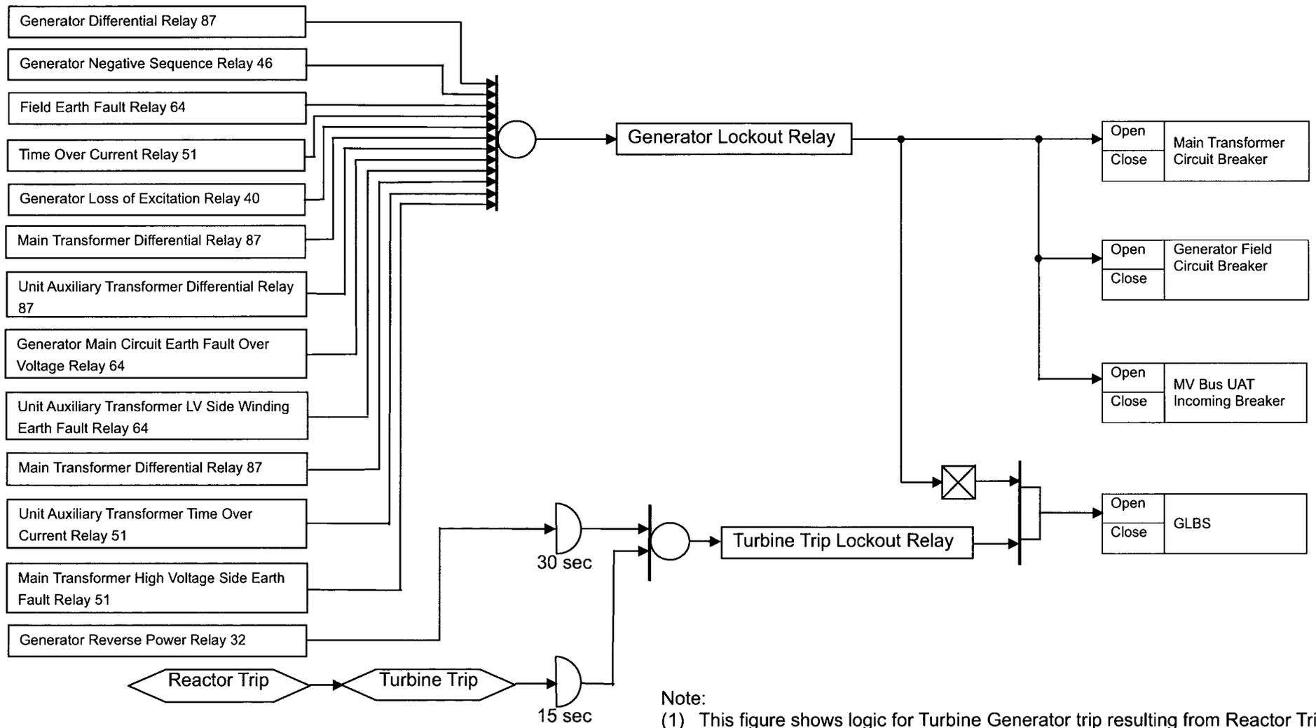
**Figure-1 Generator Circuit Interlock Diagram**
