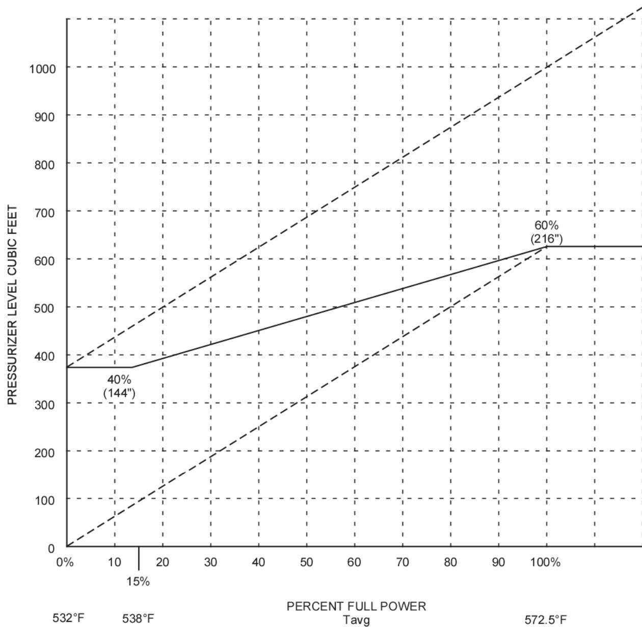
**Figure 6.2-1 Pressurizer Level Program**
