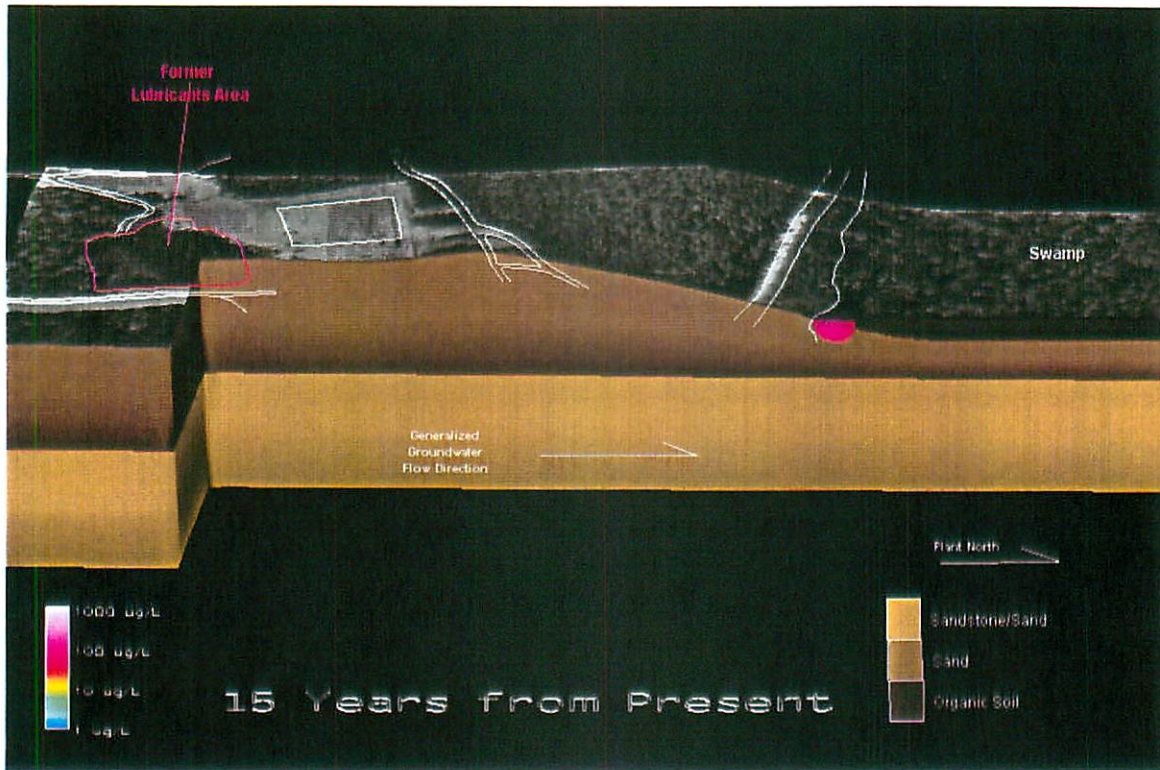
Figure 6-11 Predicted Distribution of cis-1,2 DCE (>70 µg/L) in Groundwater - 15 to 30 Years from Present - Northwest Site Area
