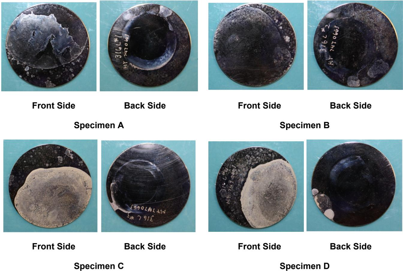
**Figure 3-1. Photos of Posttest Surfaces of 316L Stainless Steel After 37 Days of Dripping at 80 °C [176 °F] and 85 Percent Relative Humidity**
