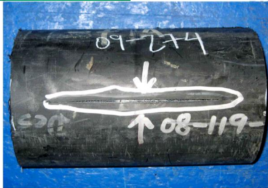
Figure 3-6 Example 3 of Pressurized Pipe Slot Failure
