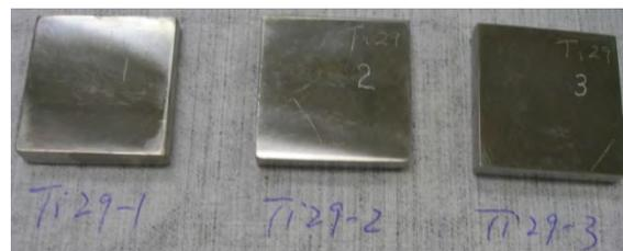
**Figure 3-18. Optical Photographs of Specimens After First HNO<sub>3</sub> Solution Cleaning Showing That Most of the Corrosion Products Were Cleaned**
