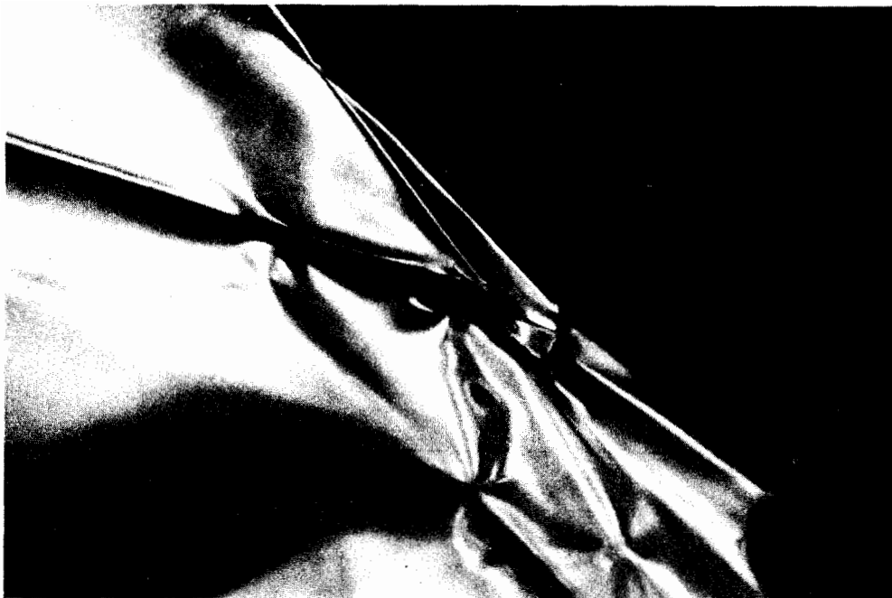
FRACTURE CAUSED BY WATER PRESSURE
