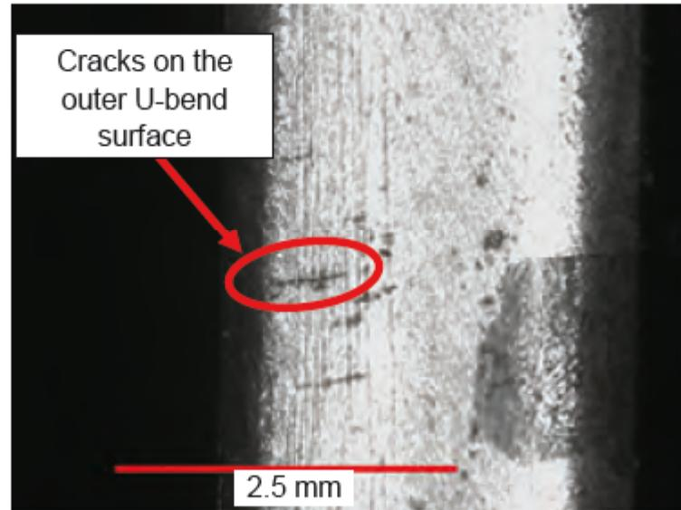
Typical SCC Behavior of a 304 Stainless Steel Single U-Bend Specimen
