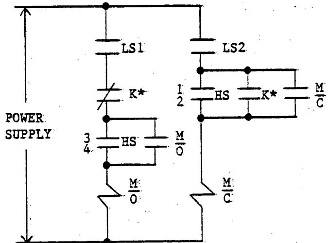
K\* Contact changes state on receipt of NSS and ES signal.
