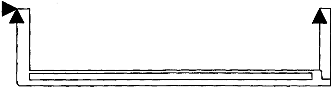
Figure 2.10.1-5a: 2D Lid End Drop - Boundary Condition
