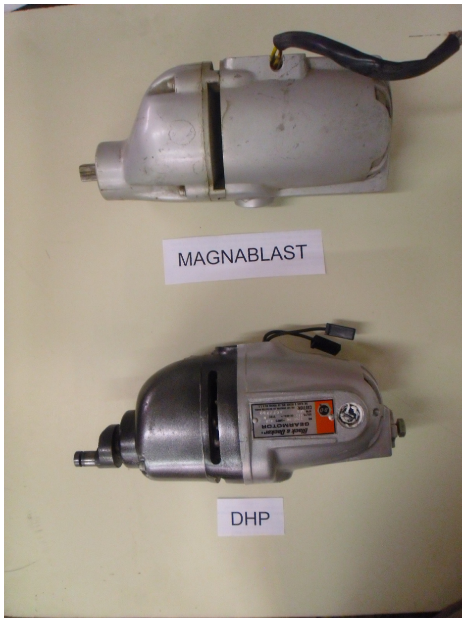
Figure 3-2 typical circuit breaker charging motor
