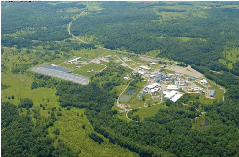
The SDA is a 15 acre State regulated pre-Part 61 shallow land disposal facility which received radioactive wastes from 1963 through 1975. There are two areas within the SDA, north and south, each consisting of seven disposal trenches. It was licensed to receive by-product material, source material, and special nuclear material. Therefore it contains considerable waste not compliant with Part 61 era LLRW regulations.
