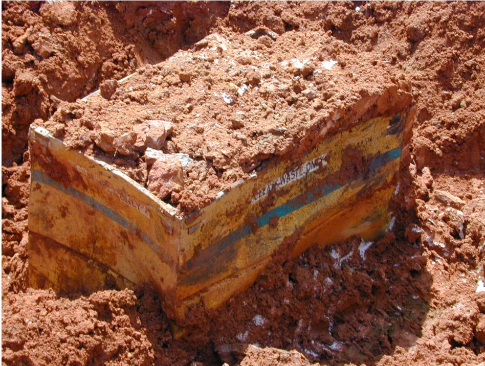
Figure 3. Exhumed Carbon Steel Box
