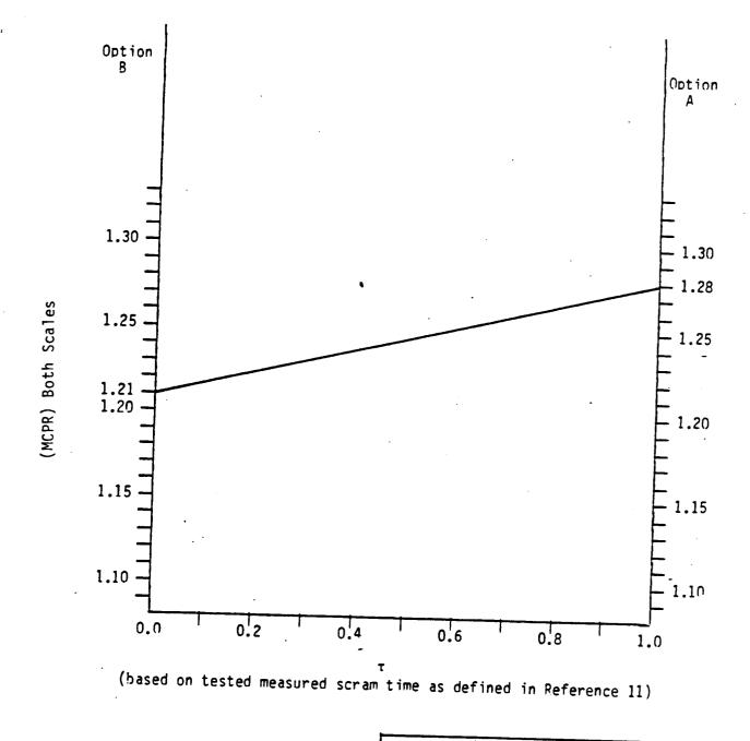
DUANE ARNOLD ENERGY CENTER IOWA ELECTRIC LIGHT AND POWER COMPANY TECHNICAL SPECIFICATIONS MINIMUM CRITICAL POWER RATIO (MCPR) VERSUS T FUEL TYPE: LTA 311 FIGURE 3.12-3
