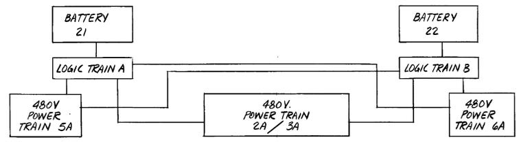
480 VOLT SYSTEM CHANNELIZATION OF LOGIC SIGNALS
