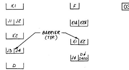
TYPICAL SECTION CABLE SPREADING ROOM
