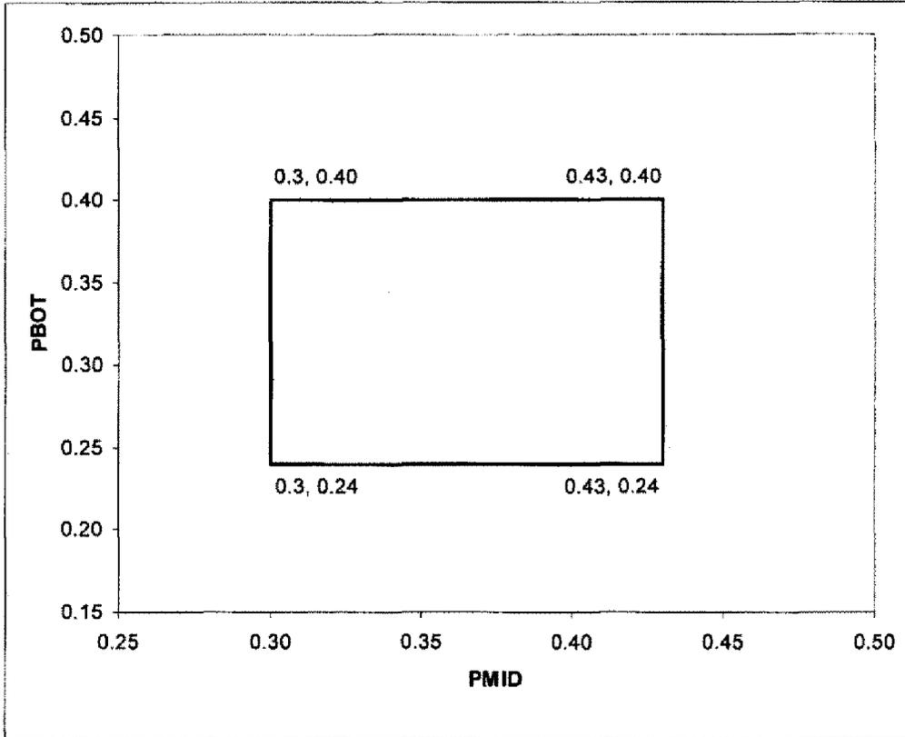
**Figure 14.3-21: Indian Point Unit 2 PBOT/PMID Analysis and Operating Limits**
