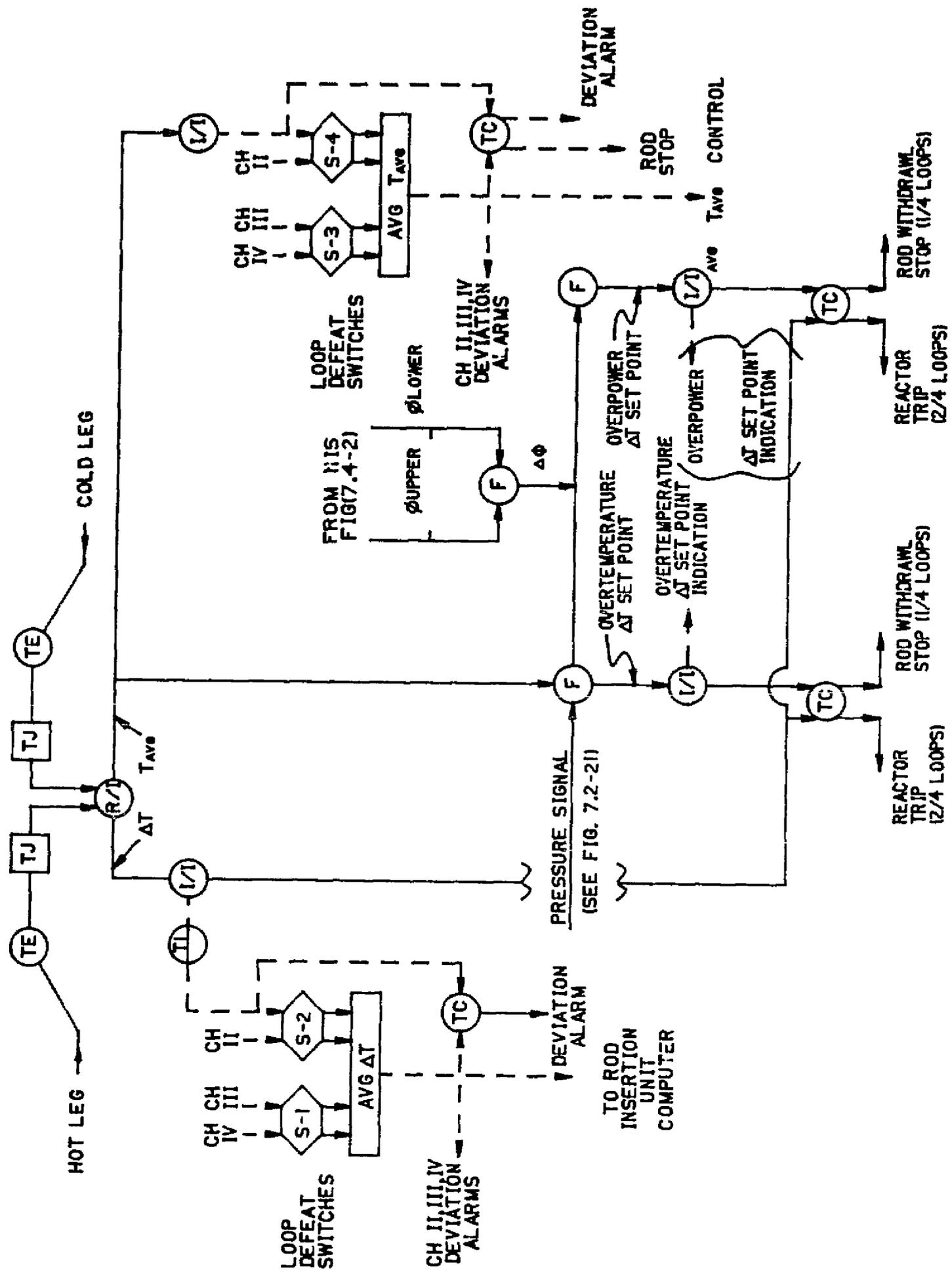
**T<sub>AVG</sub>/ΔT CONTROL AND PROTECTION SYSTEM (SINGLE CHANNEL)**
