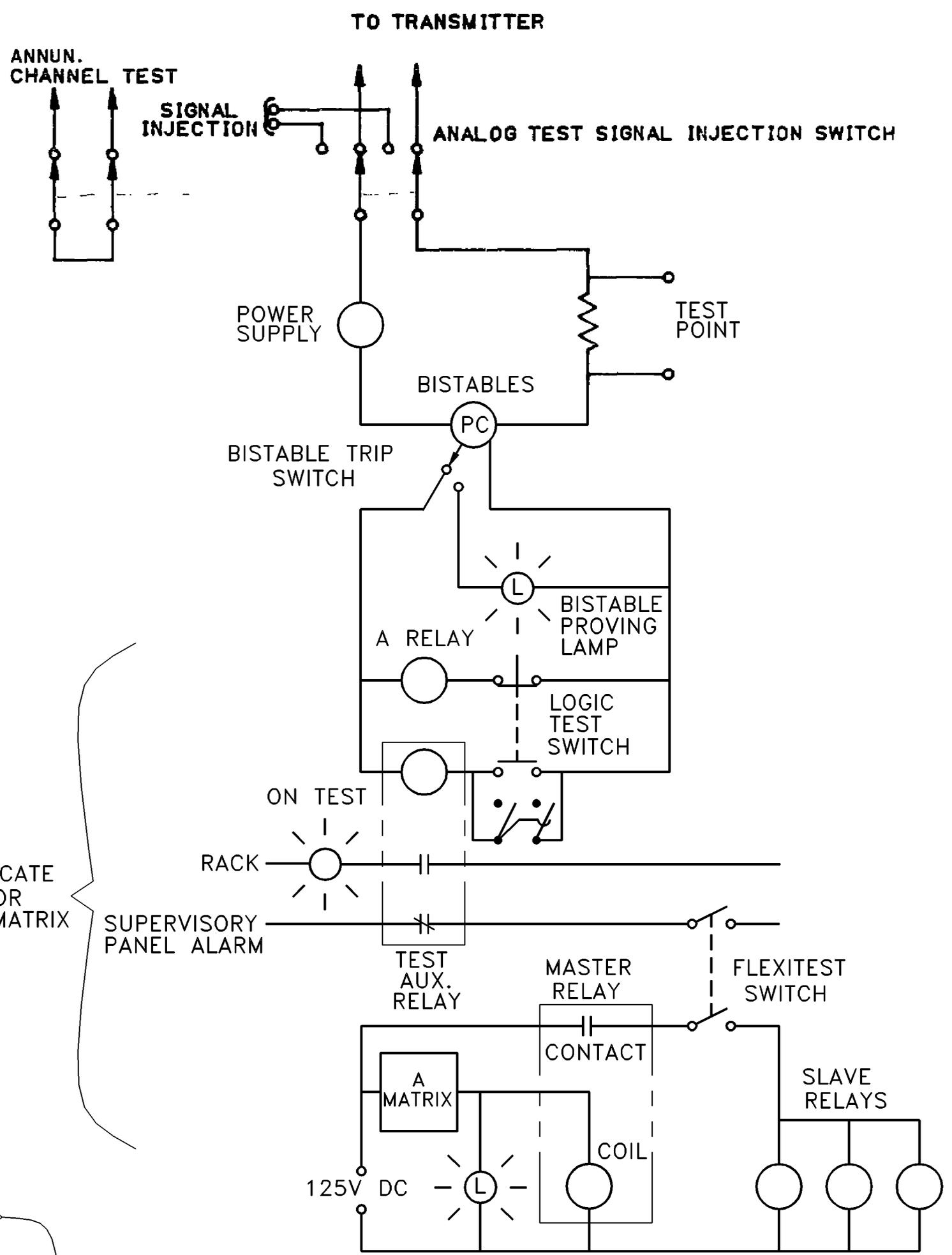
ANALOG AND LOGIC CHANNEL TESTING
