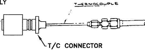
THERMOCOUPLE CONNECTOR TO
