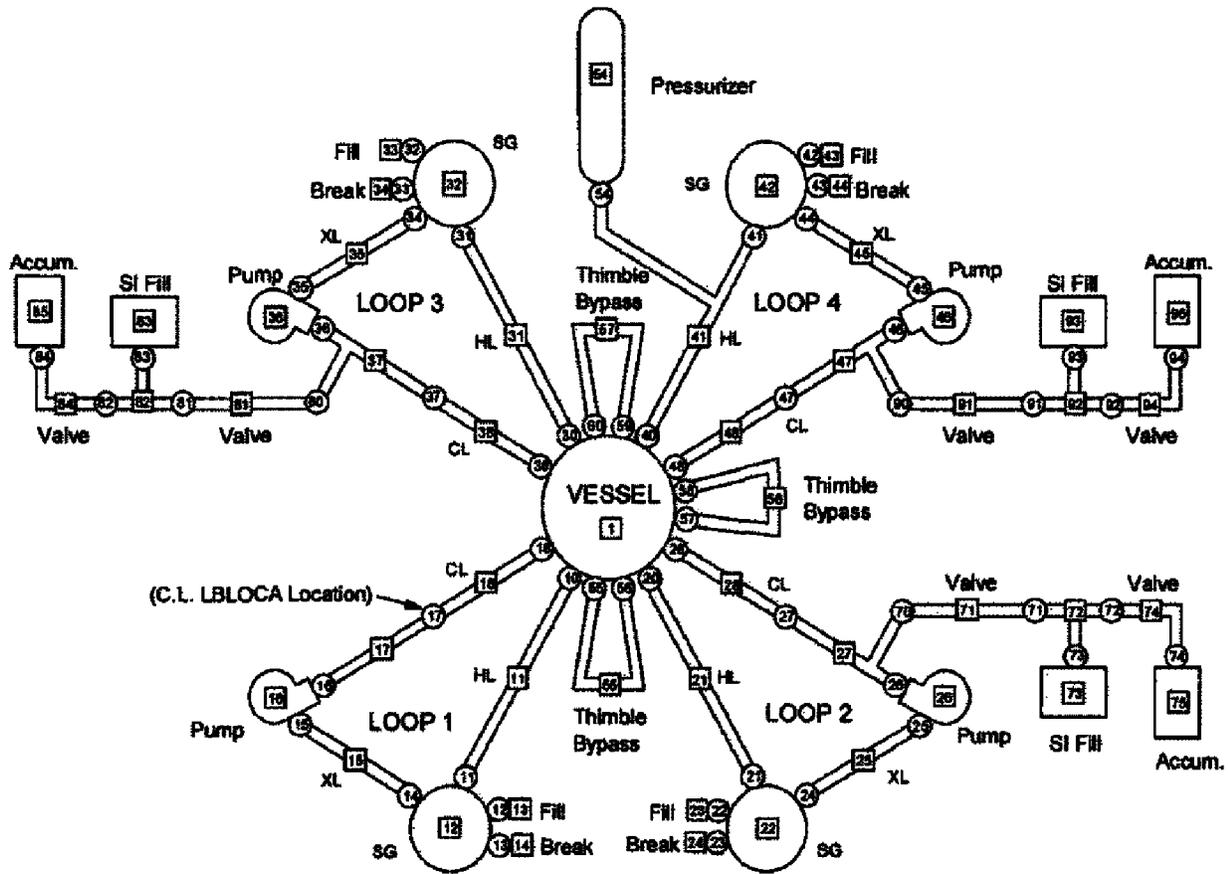
Figure 14.3-2: Indian Point Unit 2 WCOBRA/TRAC Model Loop Layout
