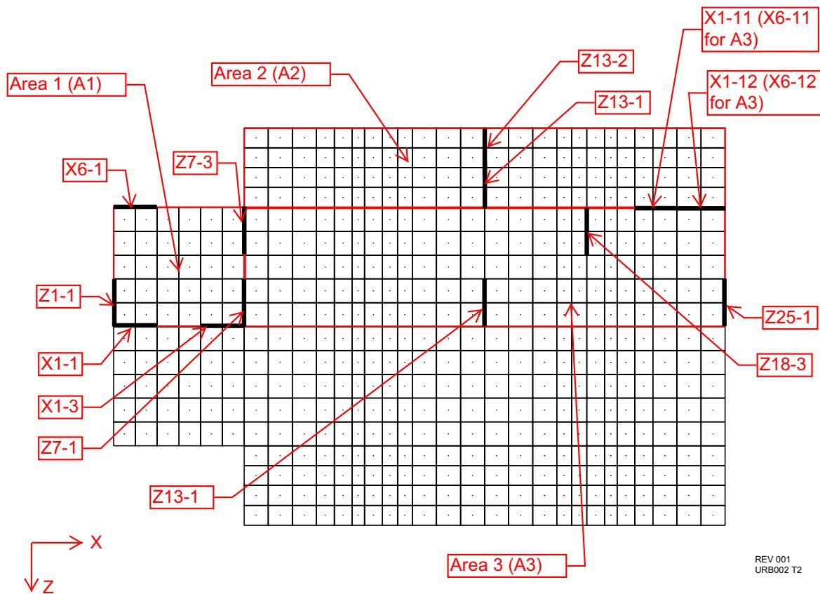
Figure 3E.3-3—Reinforcement Sketch for ESWB Basemat Foundation
