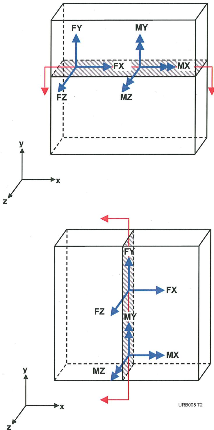
Figure 3E.3-6—Vertical and Horizontal Section Cuts for ESWB Wall at Column Line 4
