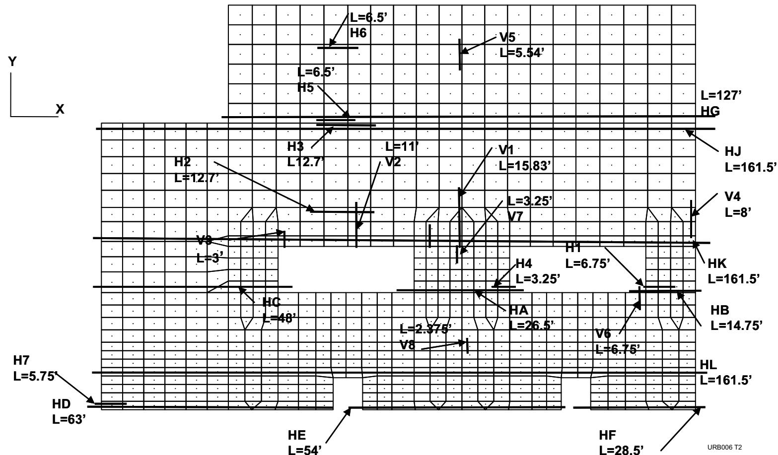
Figure 3E.3-7—Reinforcement Configuration for ESWB Wall at Column Line 4
