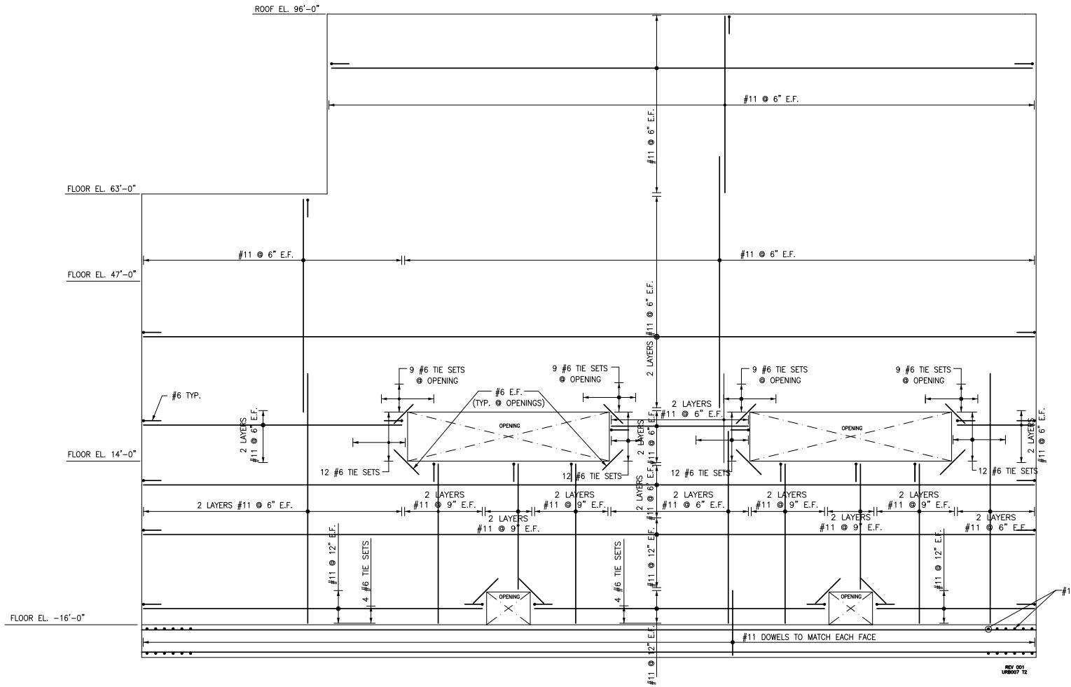
**Figure 3E.3-8—ESWB Fan Deck Slab at Elevation 63'-0" - FEM**
