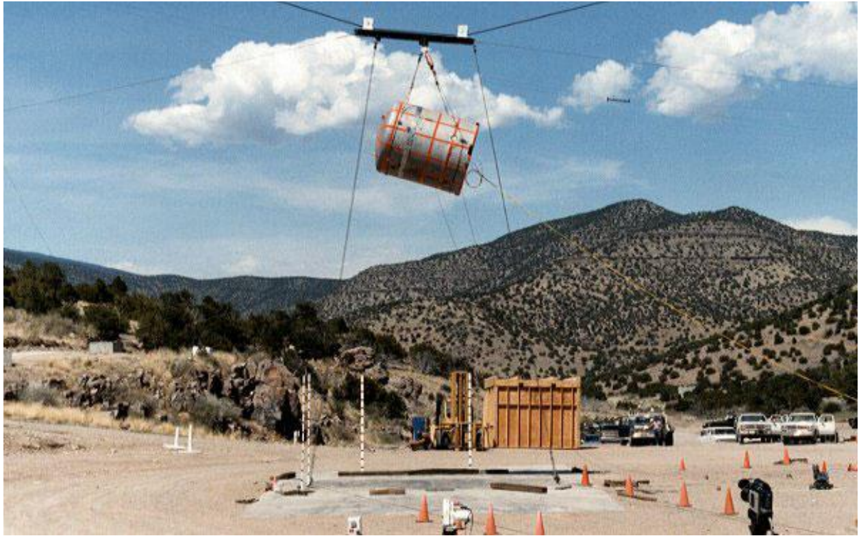
Figure 2.10.3-84 – CTU-3 Free Drop No. 3; Pre-Drop Positioning
