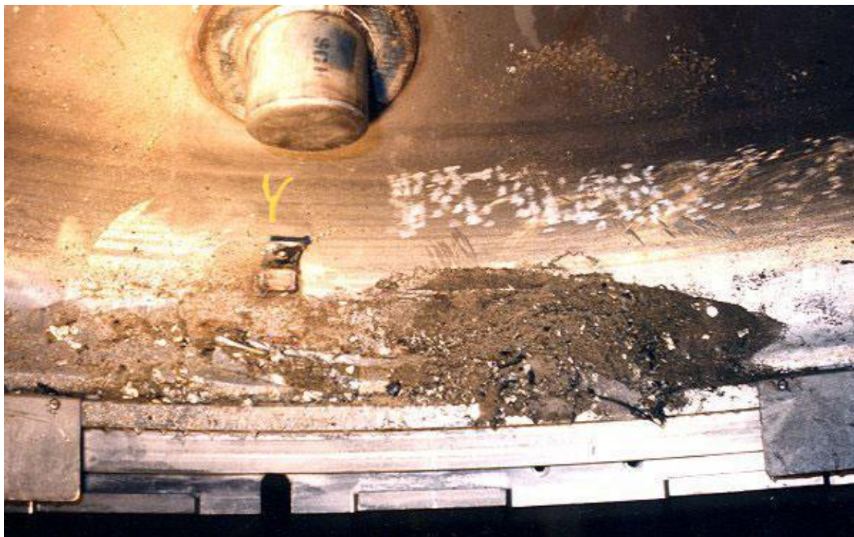
Figure 2.10.3-78 – CTU-2 Disassembly; Loose Debris in ICV Lid
