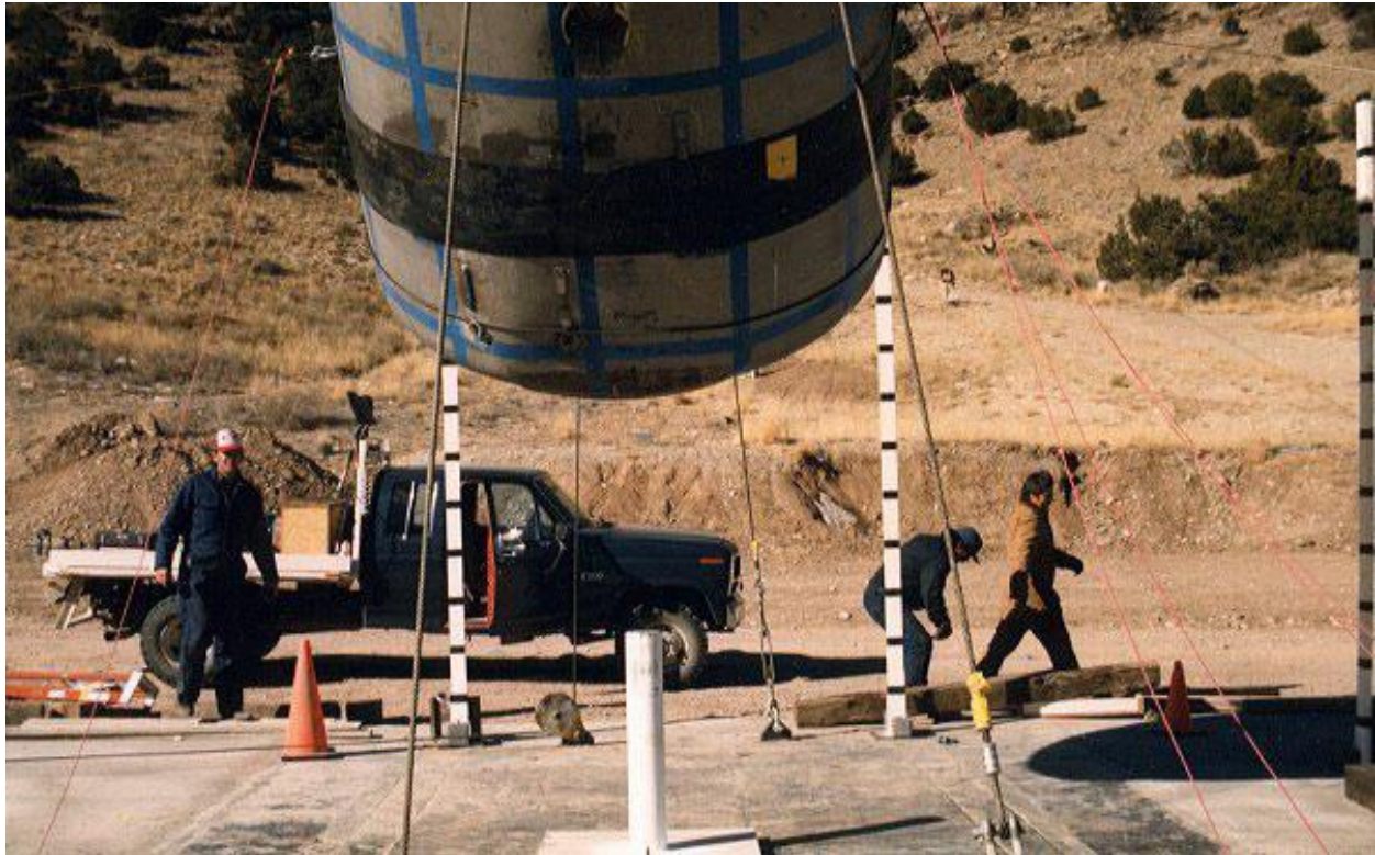
Figure 2.10.3-64 – CTU-2 Puncture Drop No. 4; Pre-Drop Positioning
