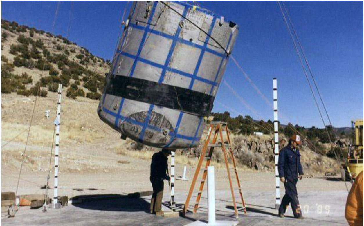
Figure 2.10.3-68 – CTU-2 Puncture Drop No. 6; Pre-Drop Positioning
