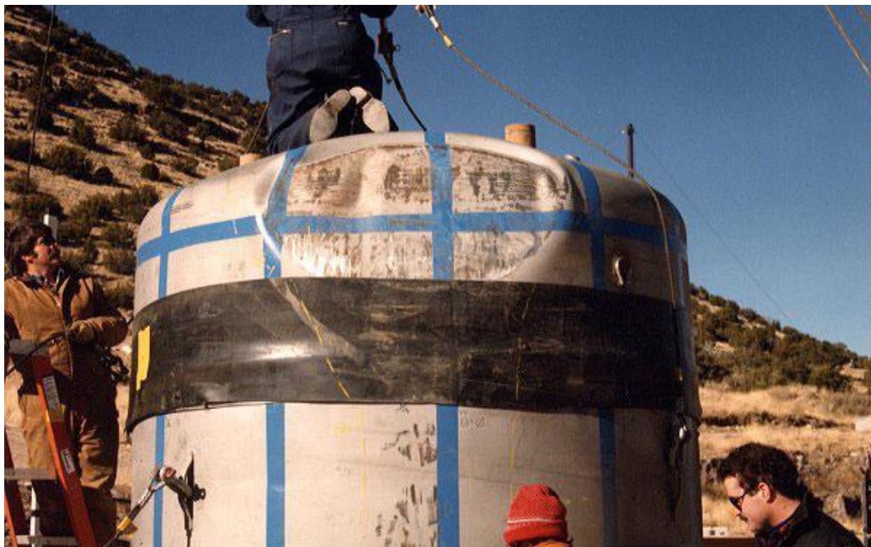
Figure 2.10.3-56 – CTU-2 Free Drop No. 1; Post-Drop Damage
