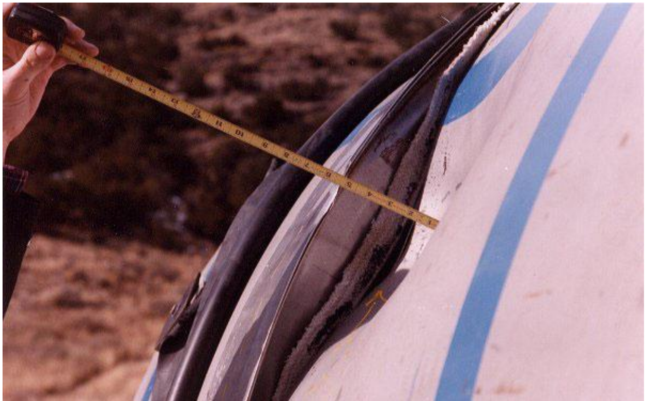
Figure 2.10.3-71 – CTU-2 Puncture Drop 7; Post-Drop Damage
