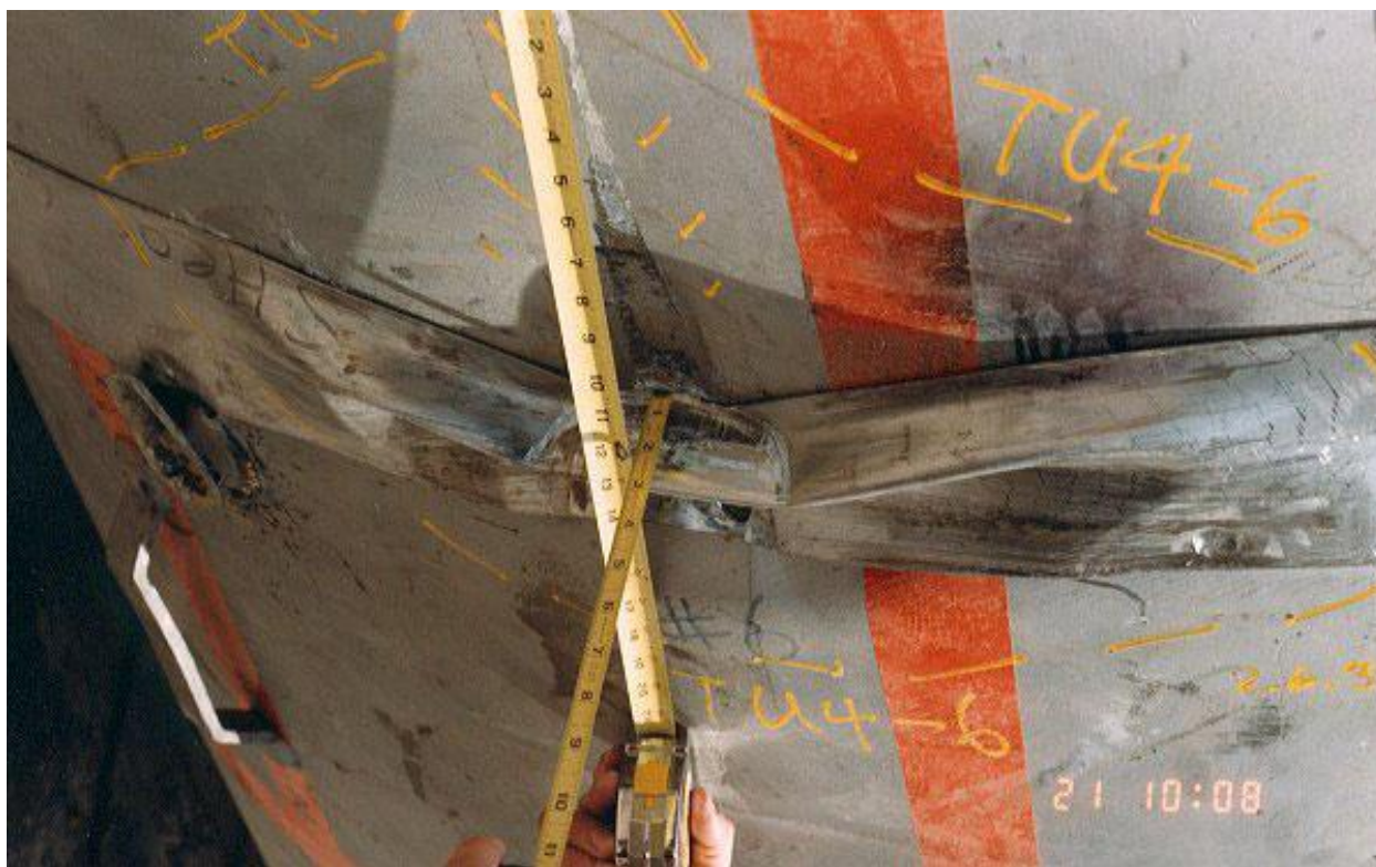
Figure 2.10.3-91 – CTU-3 Puncture Drop 6; Post-Drop Damage
