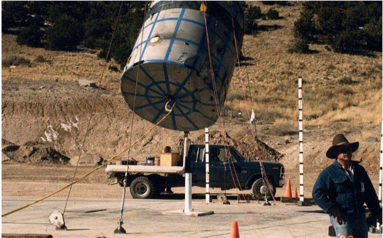
Figure 2.10.3-66 – CTU-2 Puncture Drop No. 5; Pre-Drop Positioning
