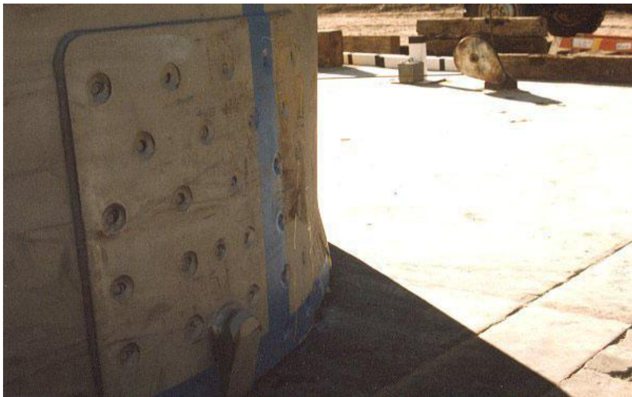
Figure 2.10.3-59 – CTU-2 Free Drop No. 2; Post-Drop Damage
