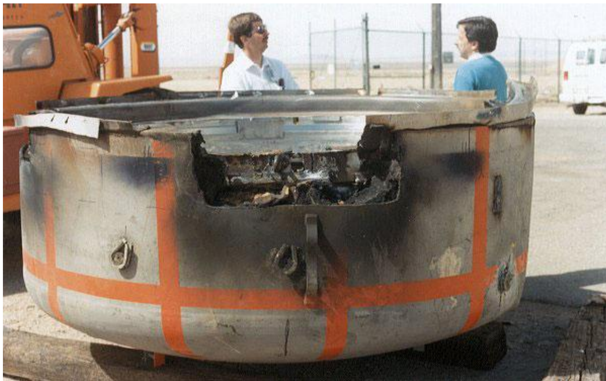
Figure 2.10.3-96 – CTU-3 Disassembly; OCA Lid
