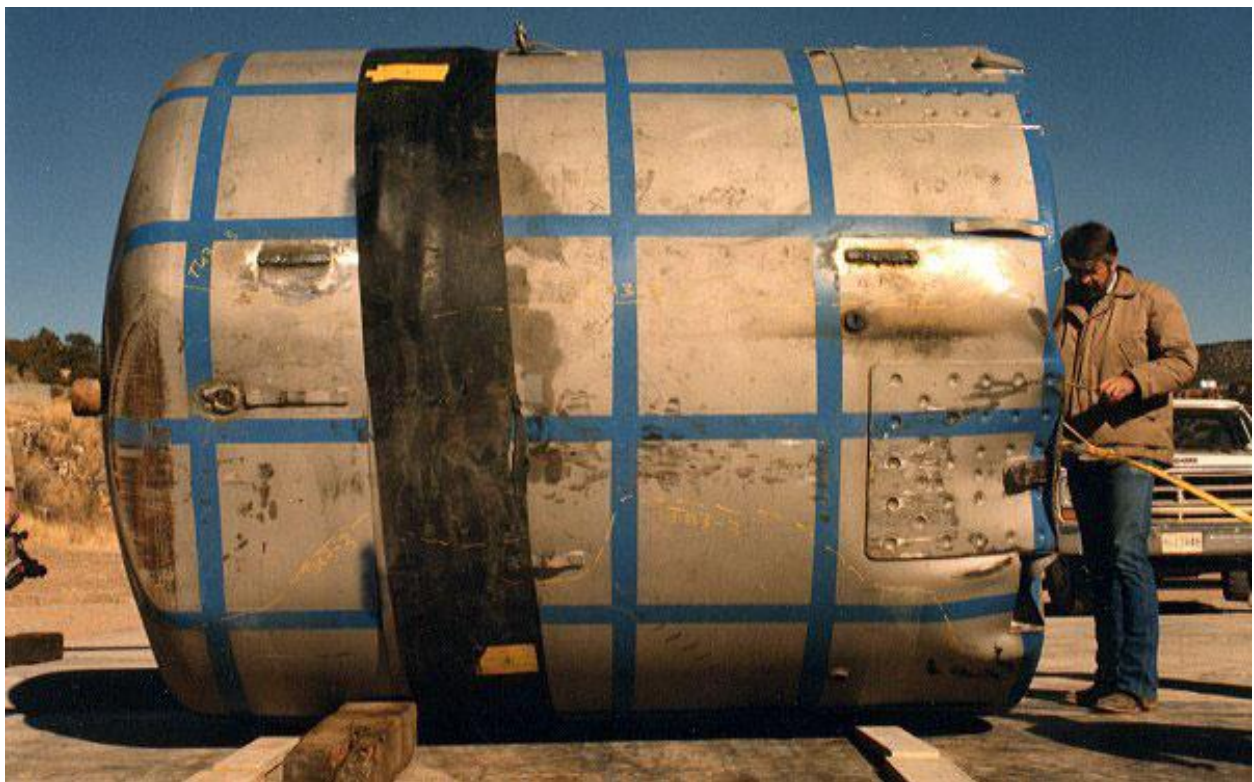
Figure 2.10.3-61 – CTU-2 Free Drop No. 3; Post-Drop Damage
