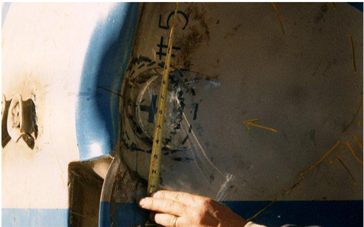
Figure 2.10.3-67 – CTU-2 Puncture Drop 5; Post-Drop Damage
