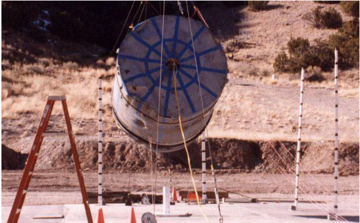
Figure 2.10.3-70 – CTU-2 Puncture Drop No. 7; Pre-Drop Positioning
