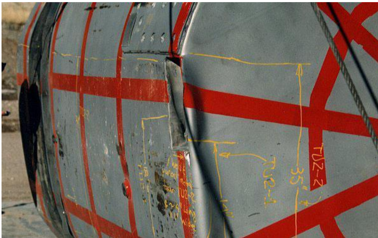
Figure 2.10.3-31 – CTU-1 Free Drop No. 2; Post-Drop Damage
