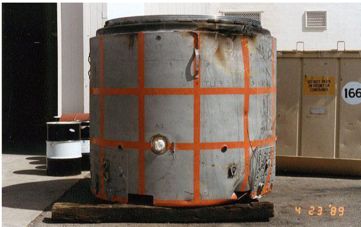
Figure 2.10.3-97 – CTU-3 Disassembly; OCA Body
