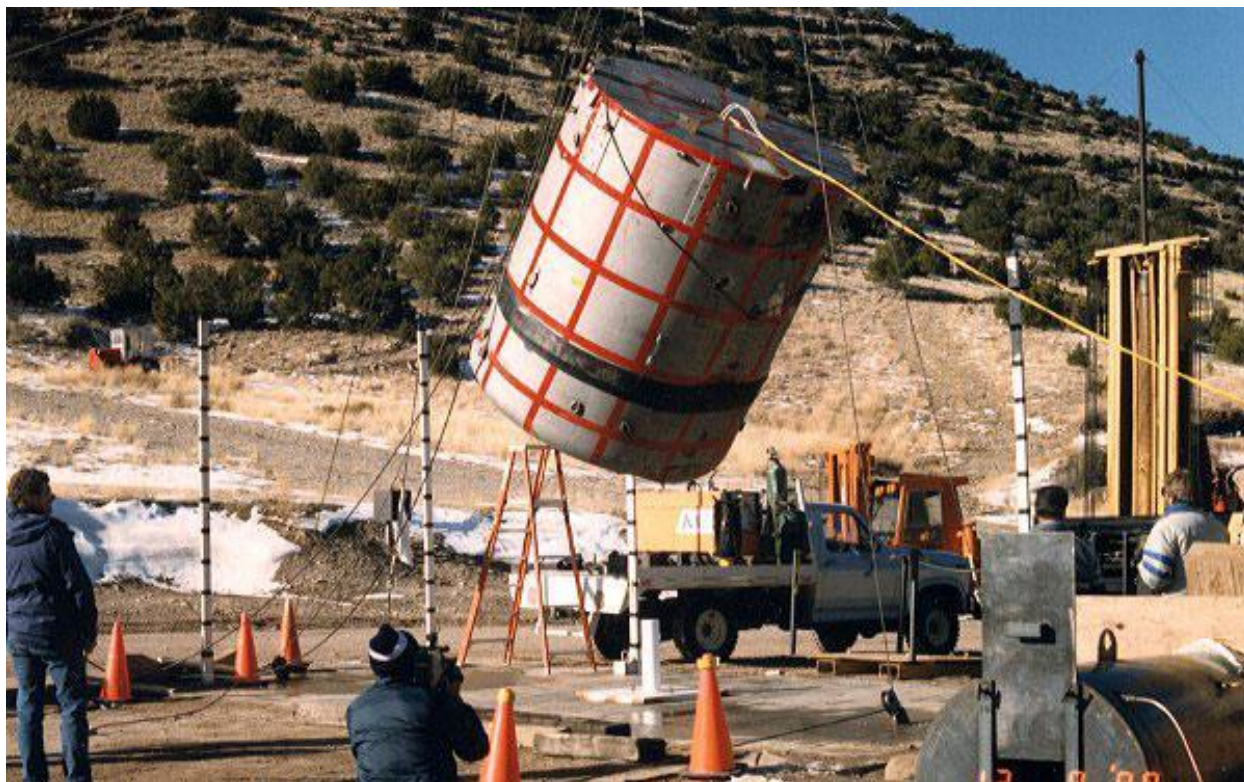
Figure 2.10.3-42 – CTU-1 Puncture Drop No. 8; Pre-Drop Positioning
