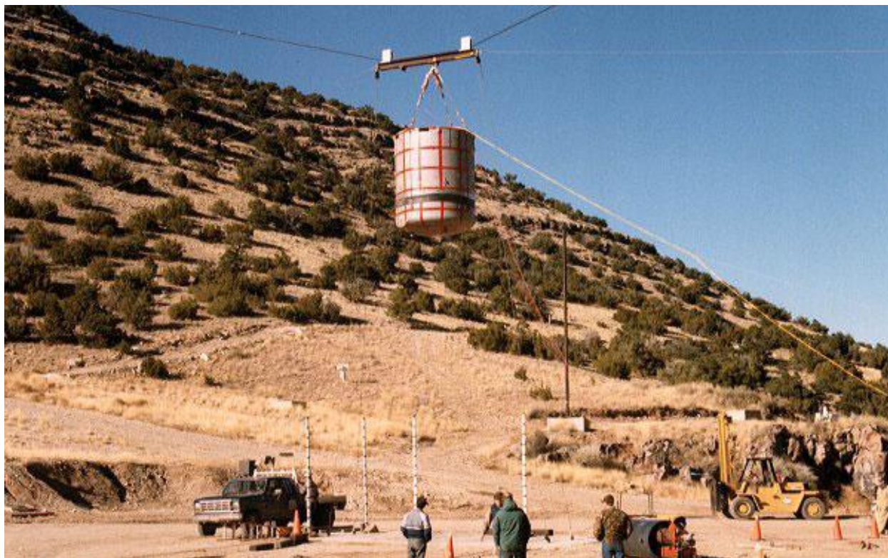
Figure 2.10.3-34 – CTU-1 Free Drop No. 4; Pre-Drop Positioning
