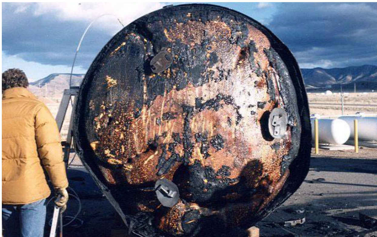
Figure 2.10.3-50 – CTU-1 Disassembly; OCA Lid Unburned Foam
