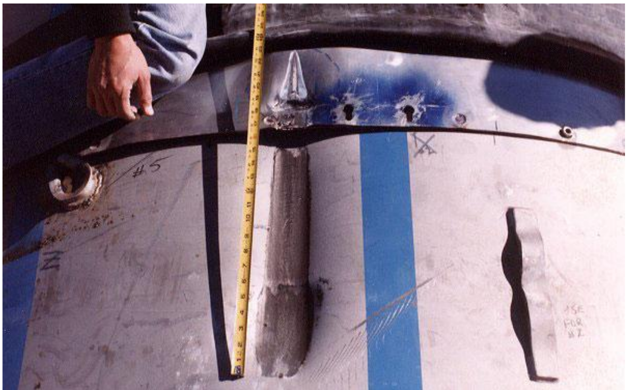
Figure 2.10.3-69 – CTU-2 Puncture Drop 6; Post-Drop Damage
