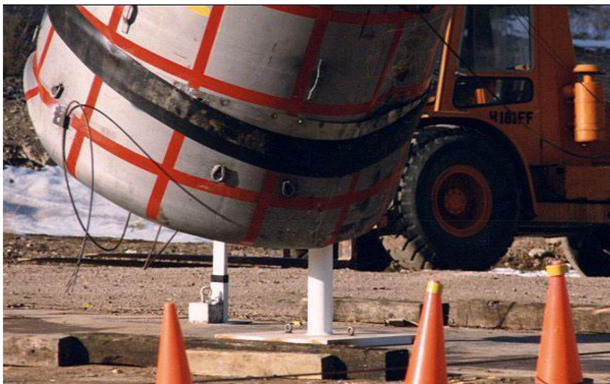
Figure 2.10.3-43 – CTU-1 Puncture Drop No. 8; Moment of Impact
