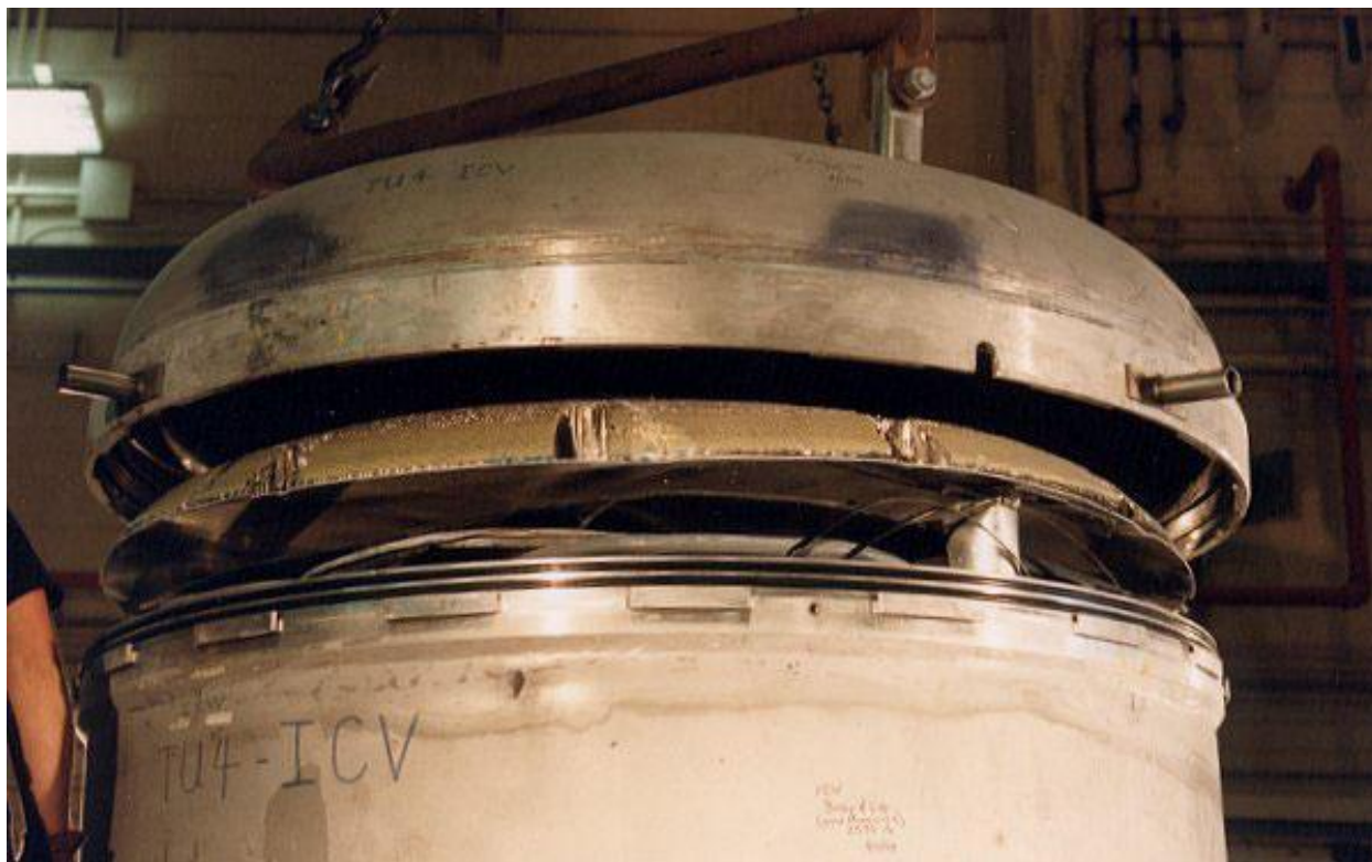
Figure 2.10.3-98 – CTU-3 Disassembly; ICV Lid Removal
