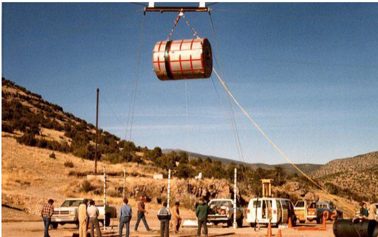
Figure 2.10.3-30 – CTU-1 Free Drop No. 2; Pre-Drop Positioning
