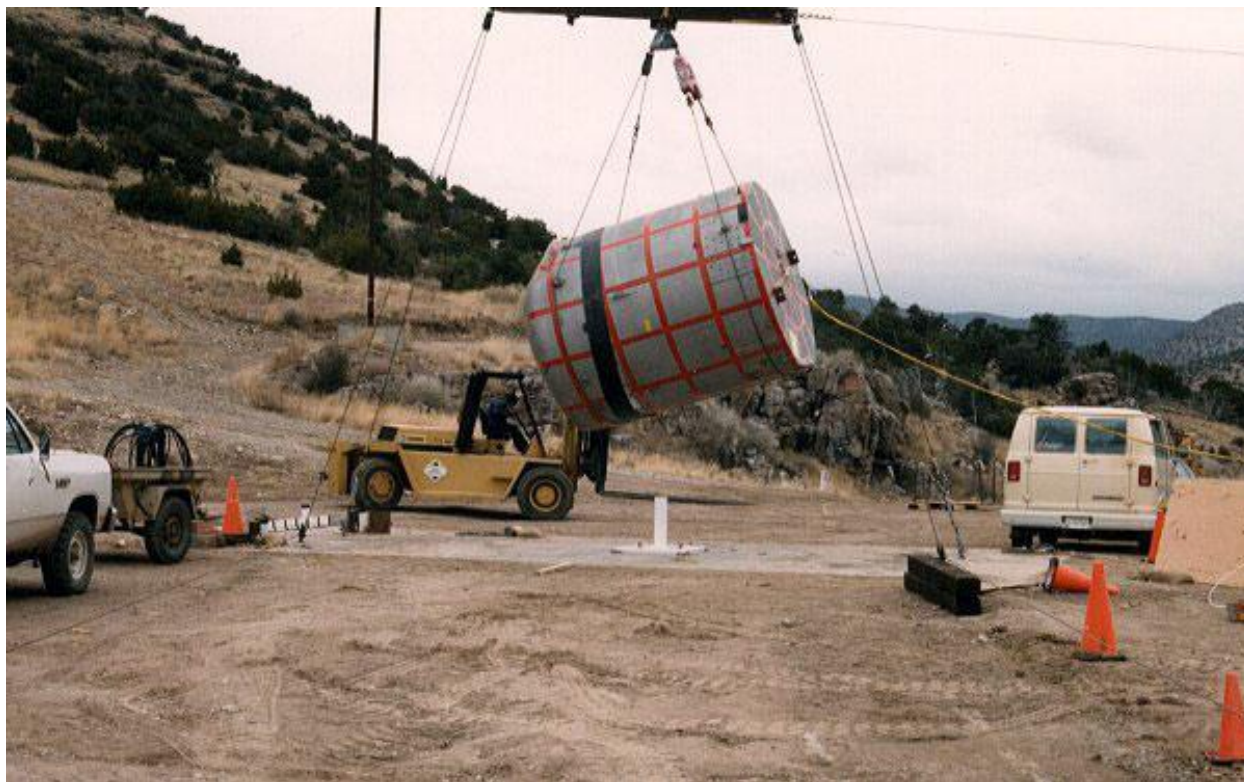
Figure 2.10.3-36 – CTU-1 Puncture Drop No. 5; Pre-Drop Positioning
