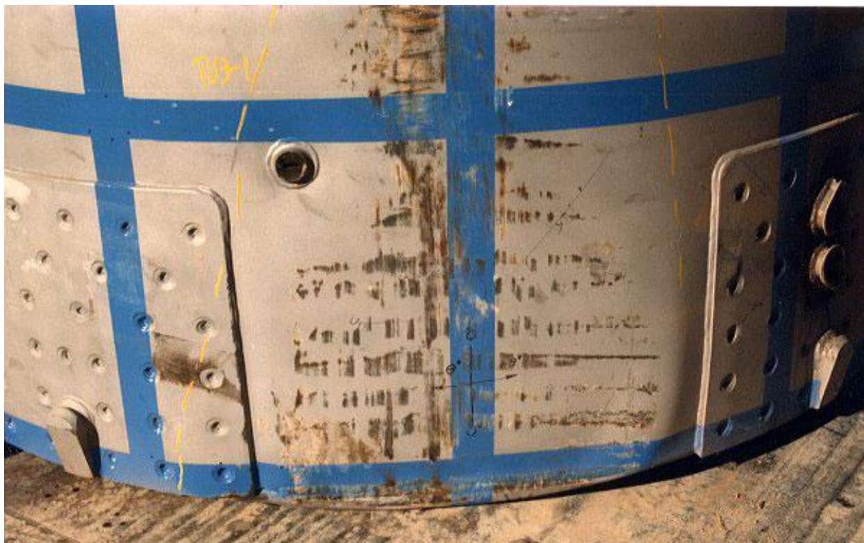
Figure 2.10.3-57 – CTU-2 Free Drop No. 1; Post-Drop Damage
