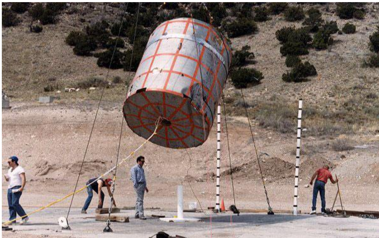
Figure 2.10.3-88 – CTU-3 Puncture Drop No. 5; Pre-Drop Positioning
