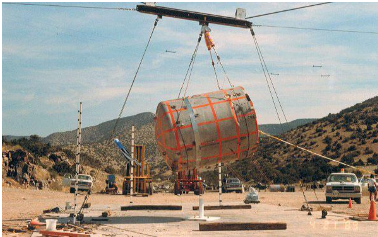
Figure 2.10.3-92 – CTU-3 Puncture Drop No. 7; Pre-Drop Positioning
