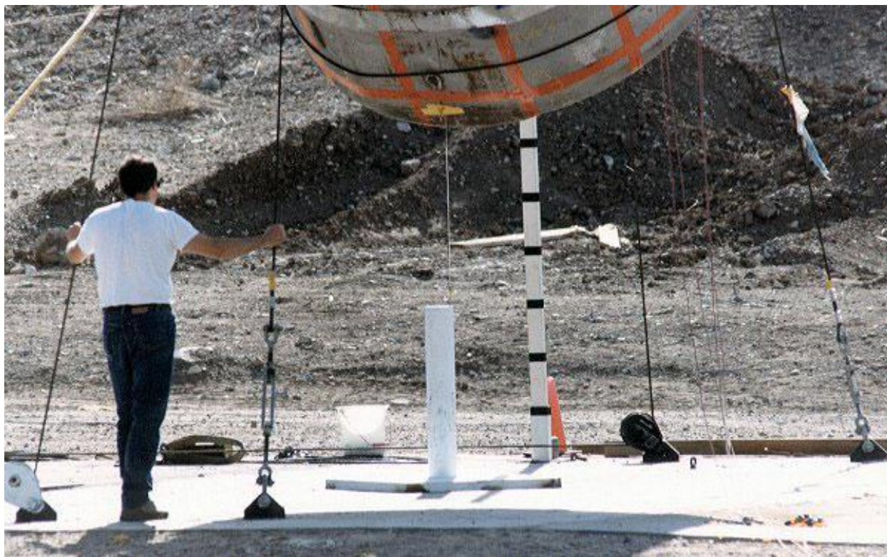
Figure 2.10.3-86 – CTU-3 Puncture Drop No. 4; Pre-Drop Positioning
