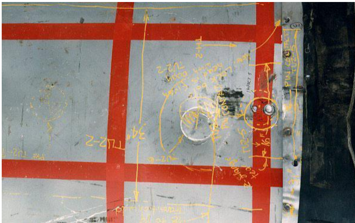
Figure 2.10.3-39 – CTU-1 Puncture Drop No. 6; Post-Drop Damage
