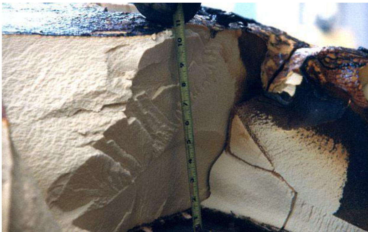
Figure 2.10.3-51 – CTU-1 Disassembly; OCA Lid Unburned Foam Thickness
