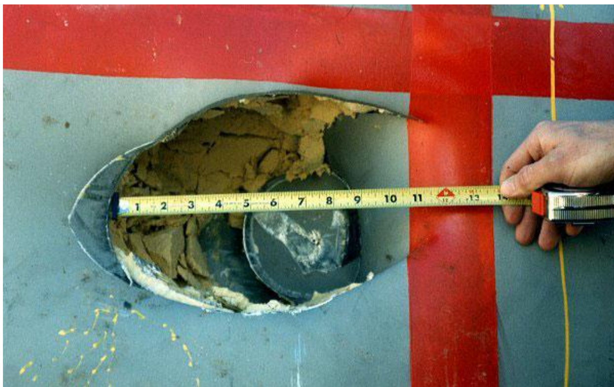
Figure 2.10.3-41 – CTU-1 Puncture Drop No. 7; Post-Drop Damage
