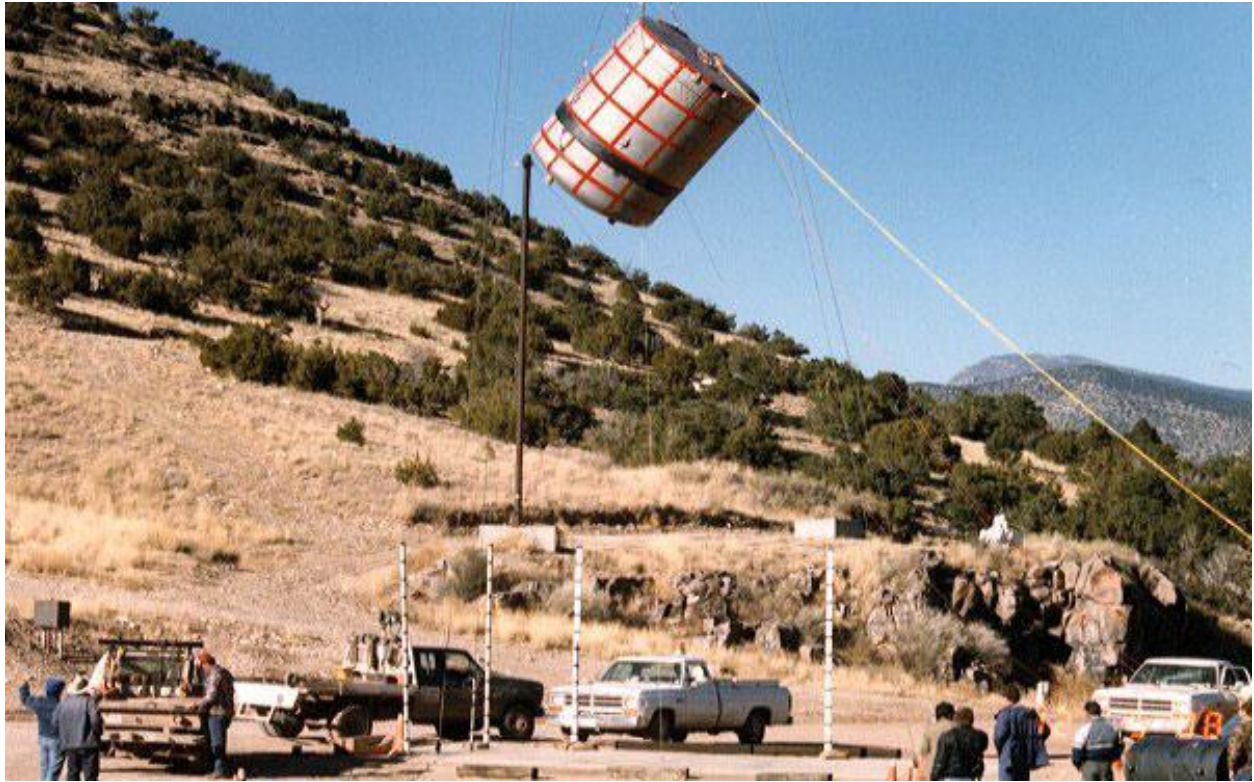
Figure 2.10.3-32 – CTU-1 Free Drop No. 3; Pre-Drop Positioning
