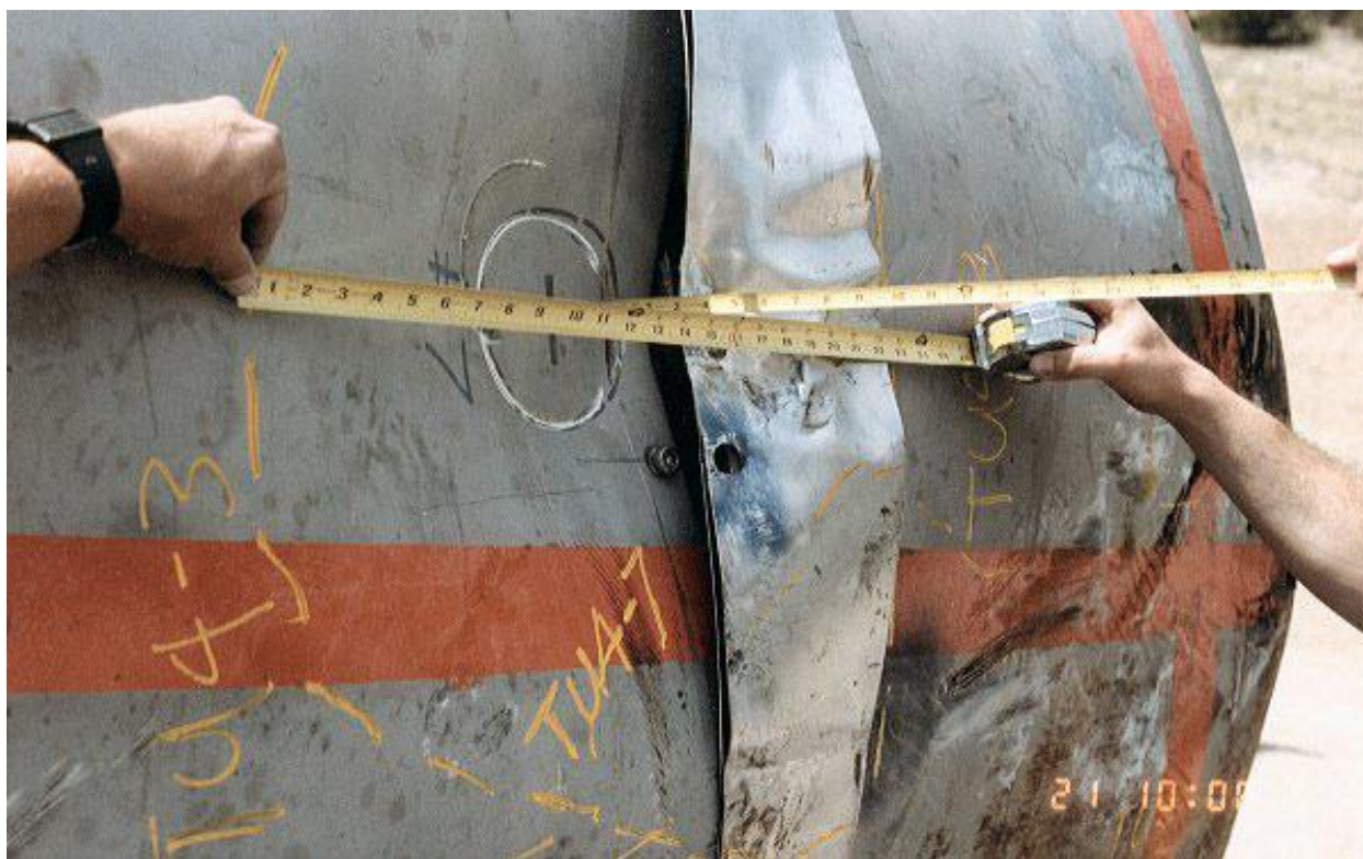
Figure 2.10.3-93 – CTU-3 Puncture Drop 7; Post-Drop Damage
