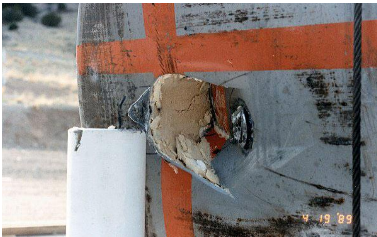
Figure 2.10.3-87 – CTU-3 Puncture Drop 4; Post-Drop Damage
