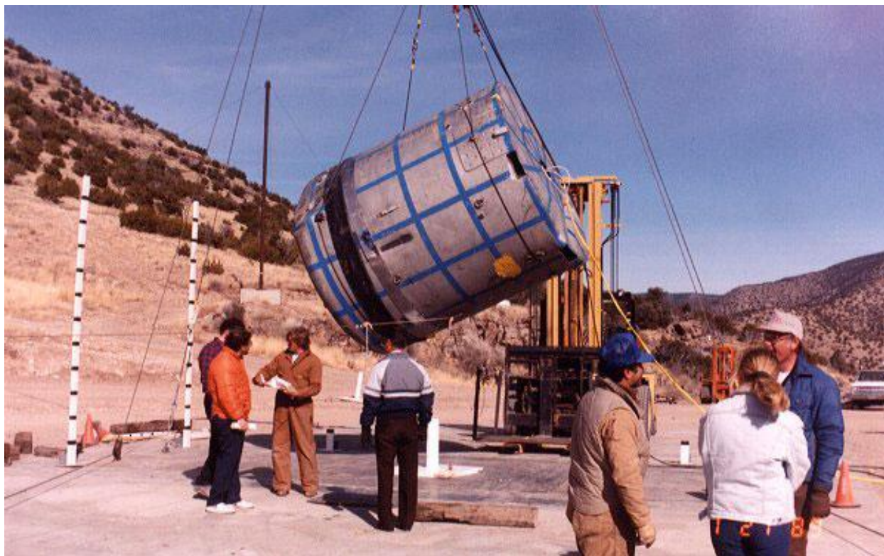
Figure 2.10.3-72 – CTU-2 Puncture Drop No. 8; Pre-Drop Positioning
