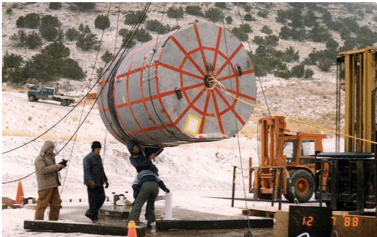
Figure 2.10.3-38 – CTU-1 Puncture Drop No. 6; Pre-Drop Positioning
