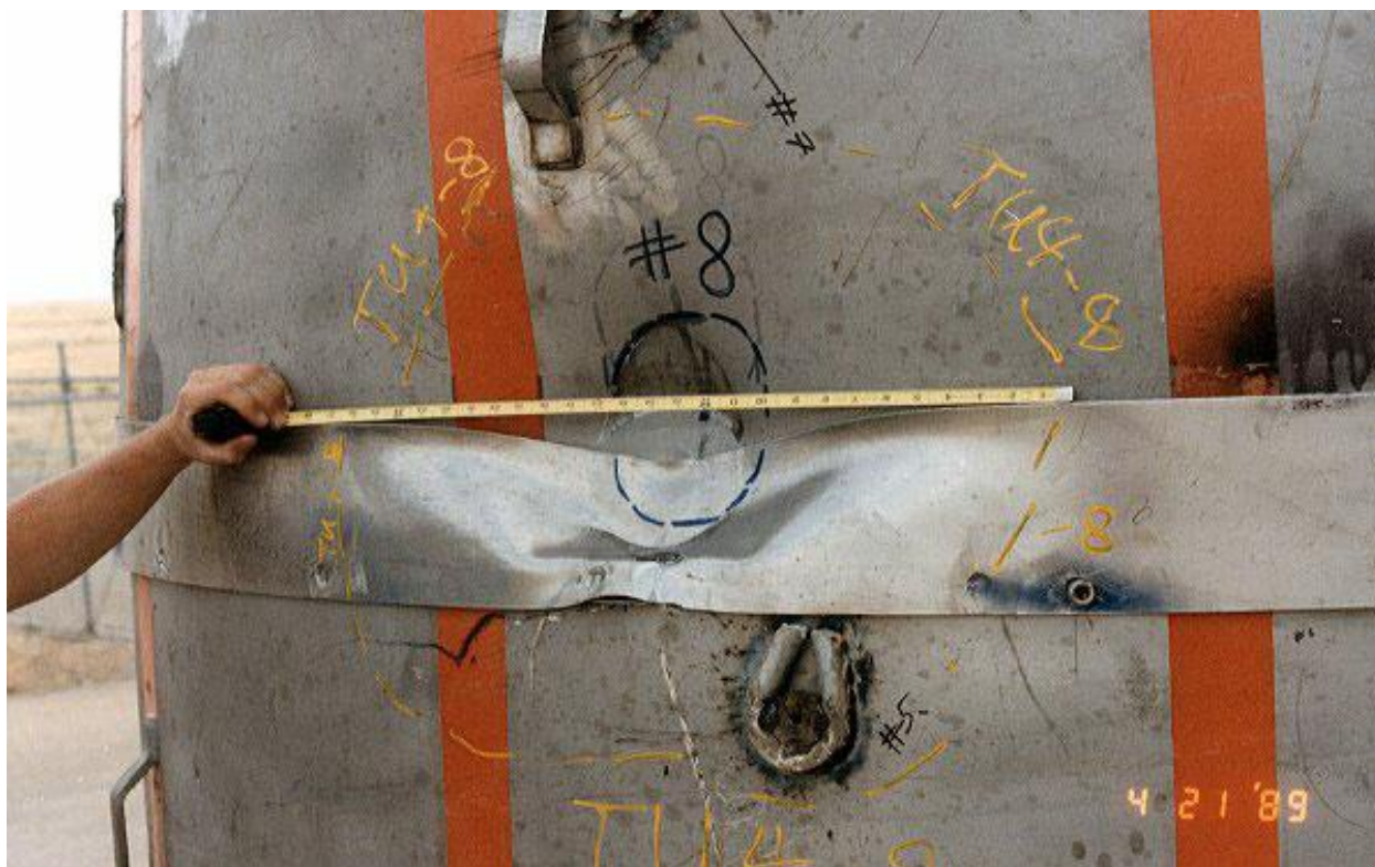
Figure 2.10.3-95 – CTU-3 Puncture Drop 8; Post-Drop Damage
