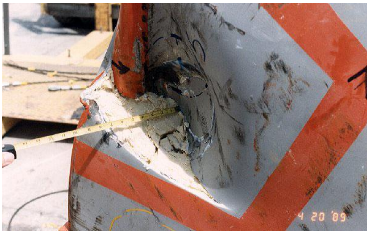
Figure 2.10.3-89 – CTU-3 Puncture Drop 5; Post-Drop Damage
