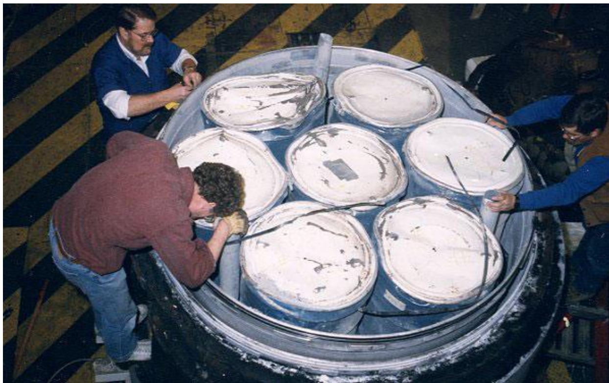
Figure 2.10.3-52 – CTU-1 Disassembly; Payload Drum Removal
