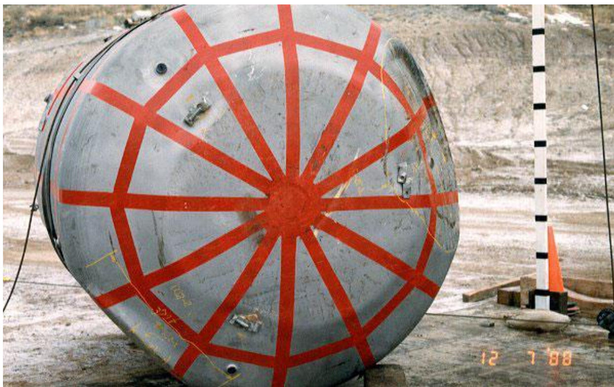
Figure 2.10.3-35 – CTU-1 Free Drop No. 4; Post-Drop Damage
