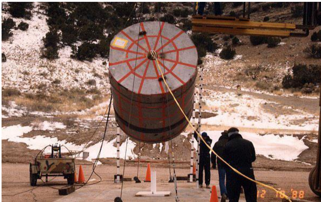
Figure 2.10.3-44 – CTU-1 Puncture Drop No. 9; Pre-Drop Positioning
