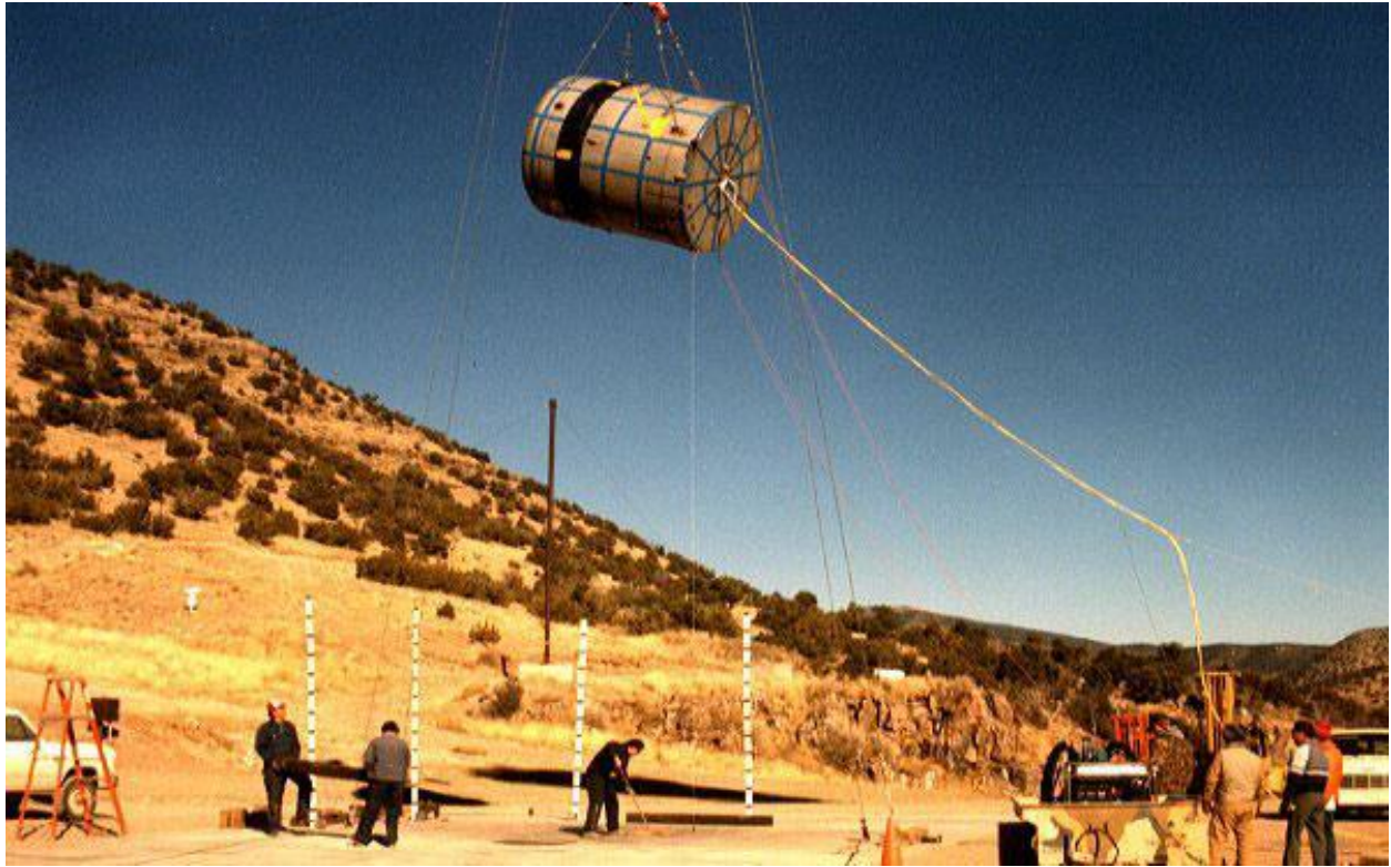
Figure 2.10.3-60 – CTU-2 Free Drop No. 3; Pre-Drop Positioning
