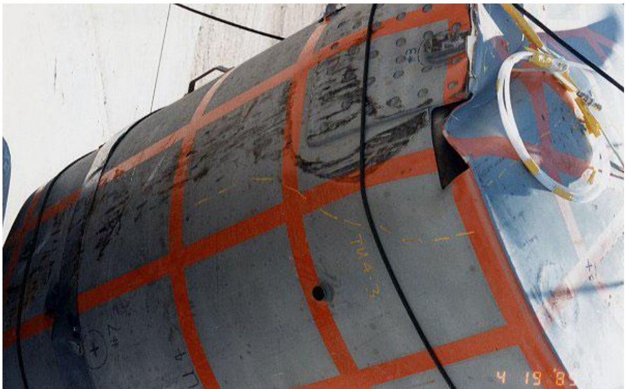
Figure 2.10.3-85 – CTU-3 Free Drop No. 3; Post-Drop Damage
