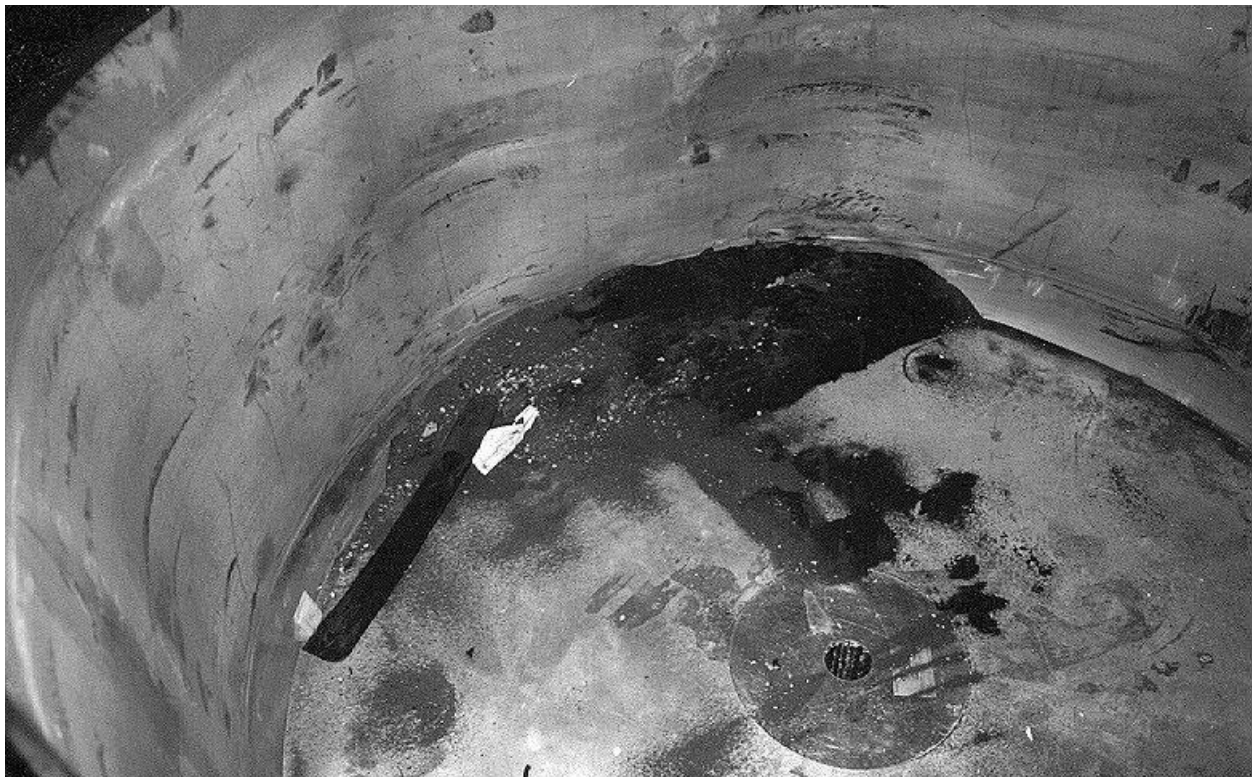
Figure 2.10.3-50 – ETU; View of Debris Inside ICV Body Cavity After Payload Drum Removal
