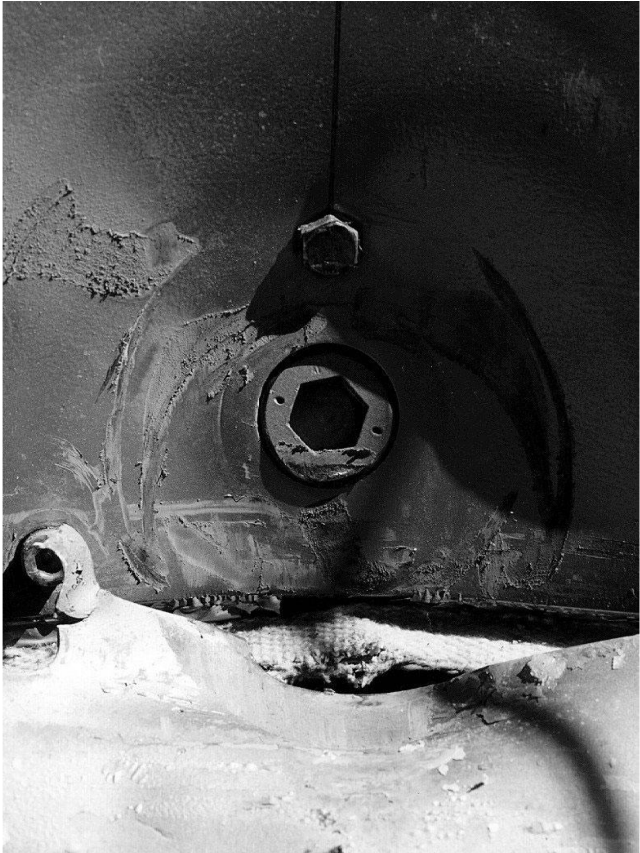
Figure 2.10.3-63 – CTU Puncture Drop Test 4; Close-up View of Damage
