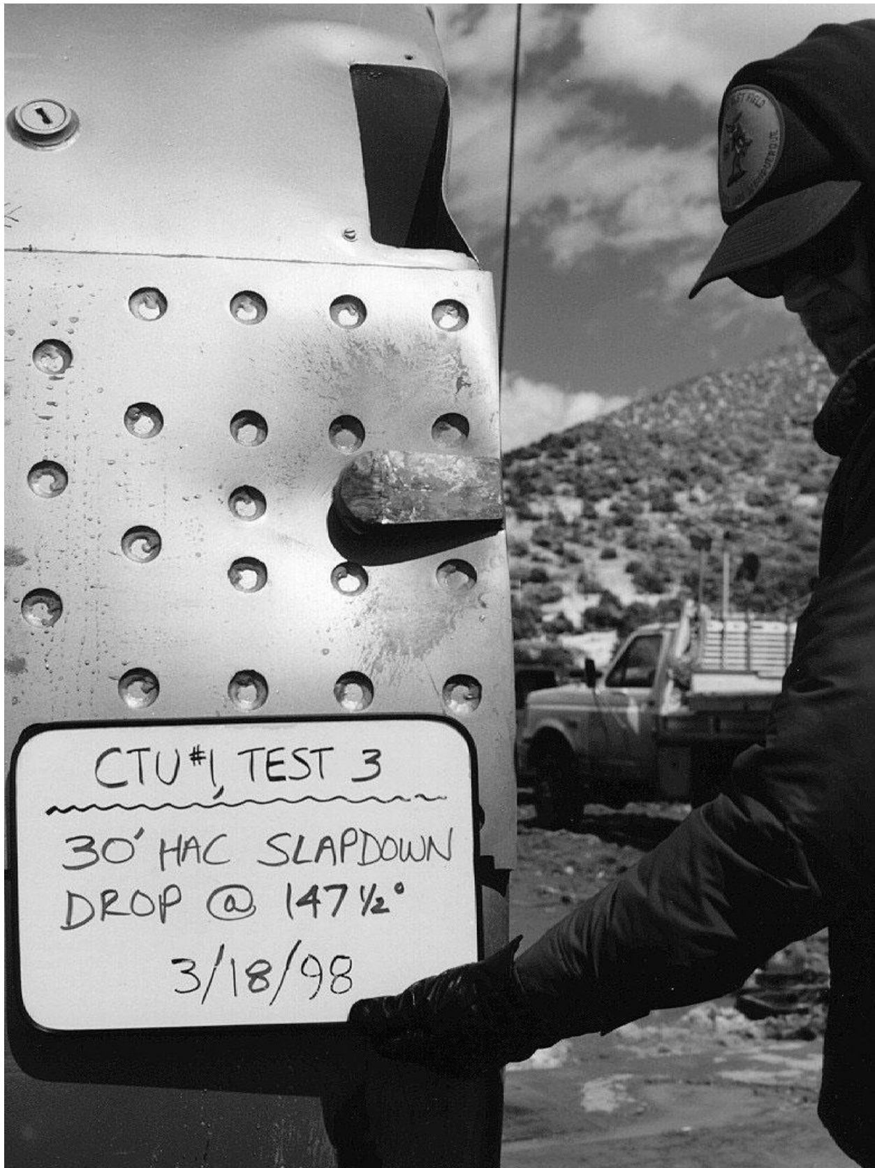
Figure 2.10.3-61 – CTU Free Drop Test 3; Bottom-End Damage
