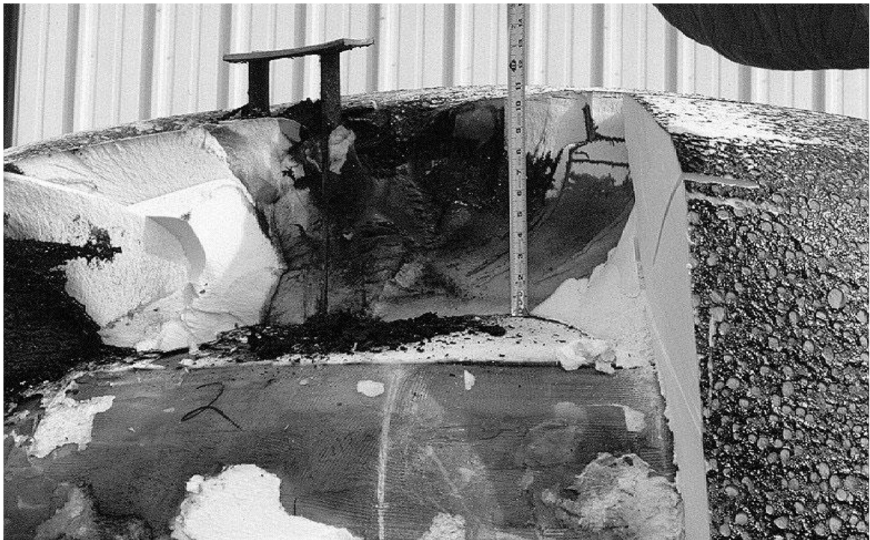
Figure 2.10.3-44 – ETU; Residual Foam in OCA Lid Top (~11")
