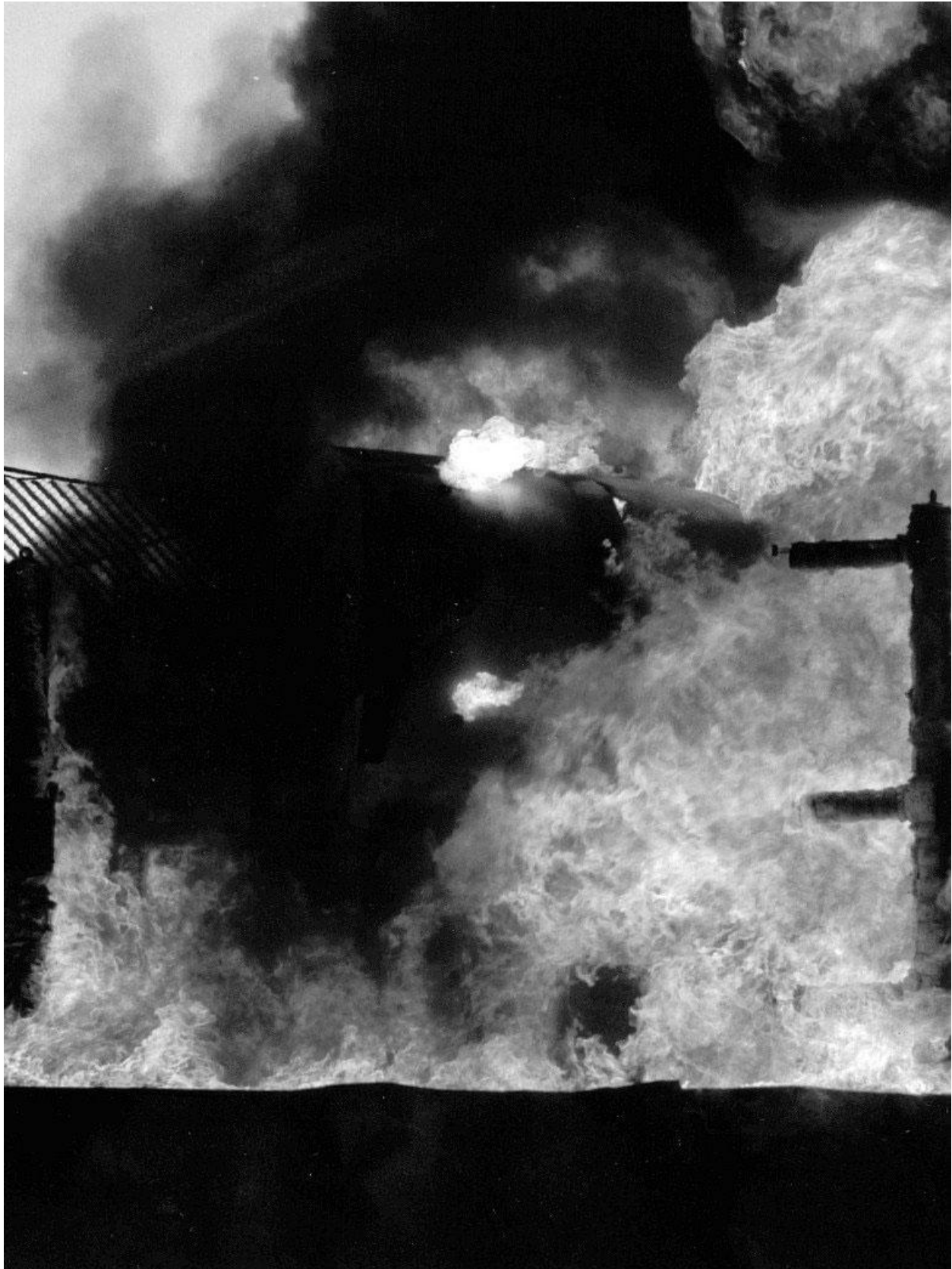
Figure 2.10.3-74 – CTU Fire Test 7; View ~28 Minutes after Start (Note Flares at Vents)
