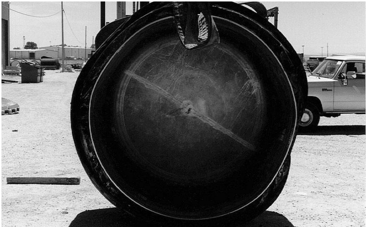
Figure 2.10.3-89 – CTU; End View of OCV Cavity Showing Deformed Lower Seal Flange
