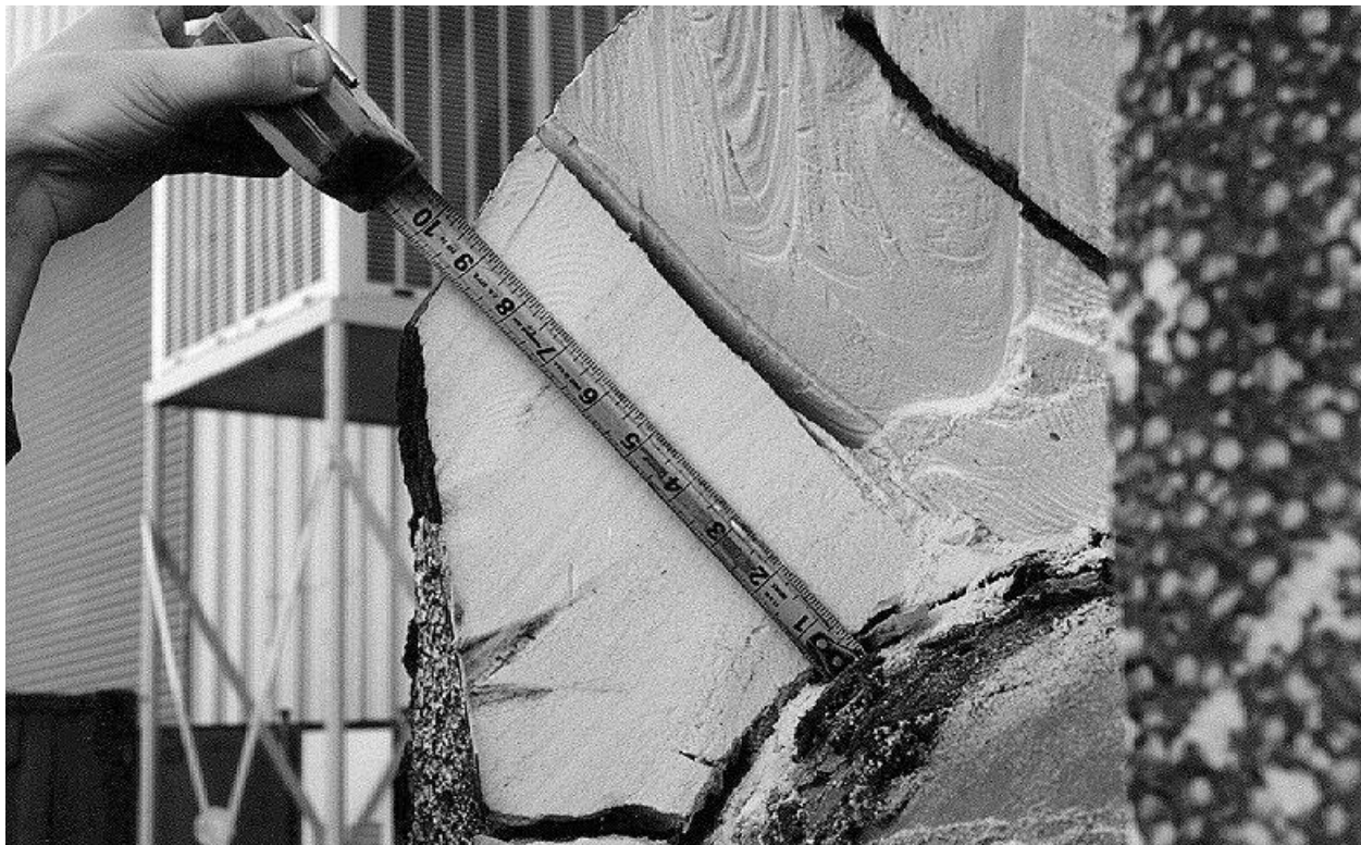
Figure 2.10.3-81 – CTU; Residual Foam in OCA Lid Knuckle; Aligned with Test 1, 2, & 4 Damage
