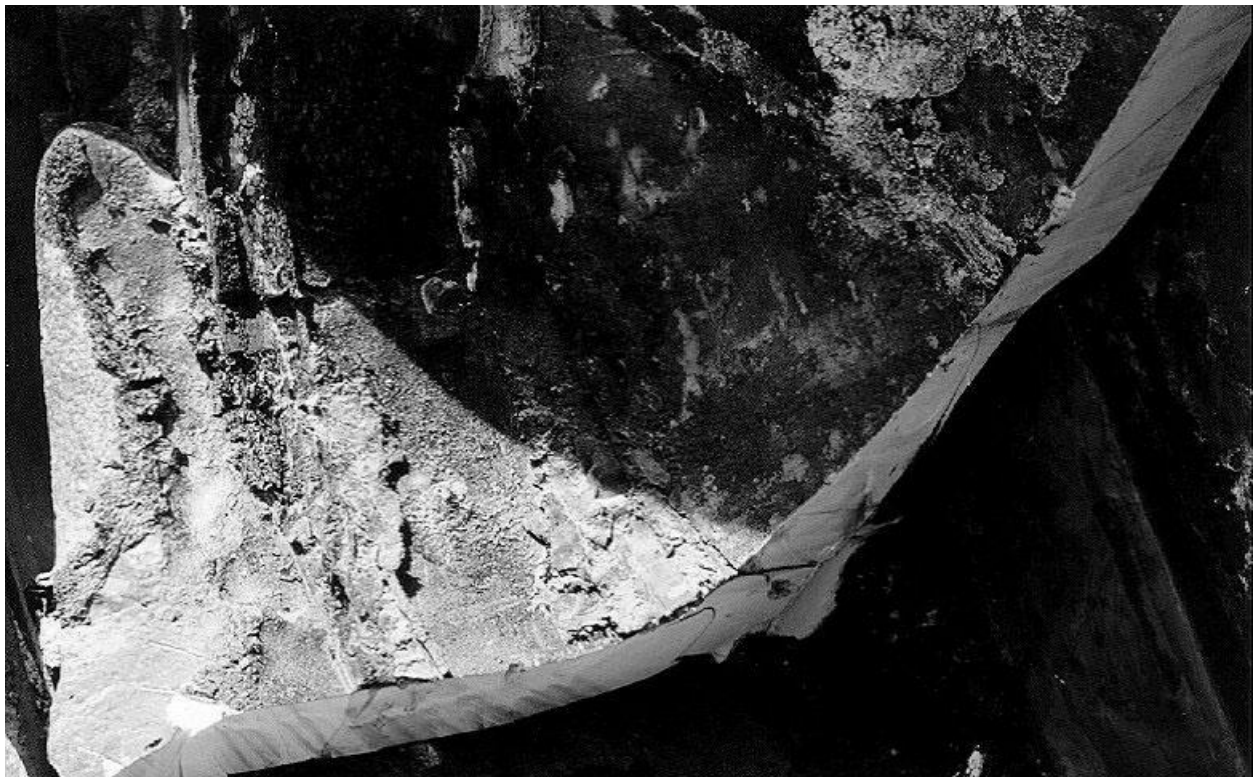
Figure 2.10.3-91 – CTU; Residual Foam in OCA Body Side; Remote from Test Damage
