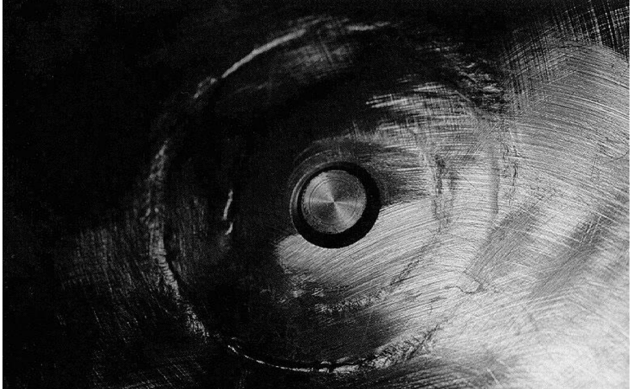
Figure 2.10.3-94 – CTU; Close-up View of Cracked OCV Vent Port Coupling Inner Weld
