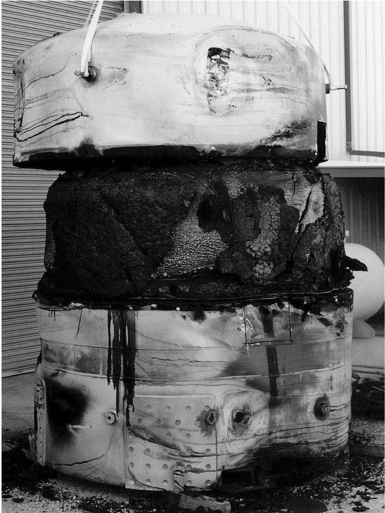
Figure 2.10.3-79 – CTU; Removal of the OCA Lid Outer Shell (Note Crumbling Foam Char)
