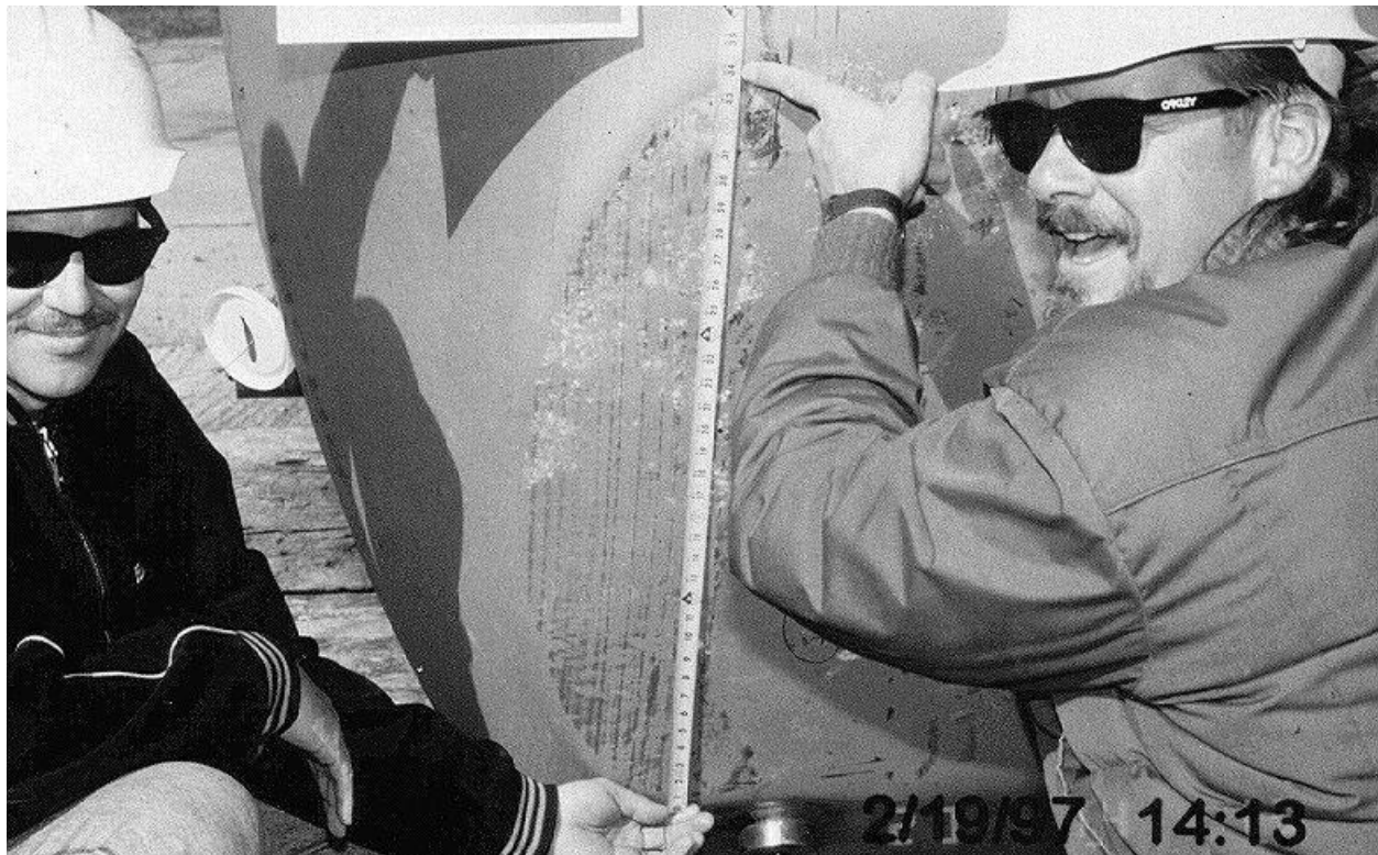
Figure 2.10.3-18 – ETU Free Drop Test 4; Top-End Damage; ~34" Wide Flat
