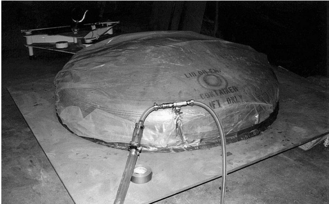
Figure 2.10.3-92 – CTU; Helium Leakage Rate Testing the ICV Lid Structure
