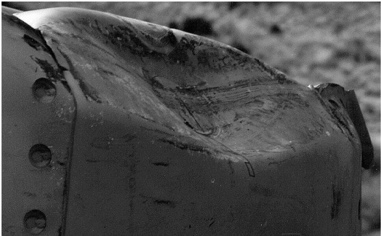
Figure 2.10.3-29 – ETU Puncture Drop Test 9; Bottom Corner Damage; ~3" Deep Dent
