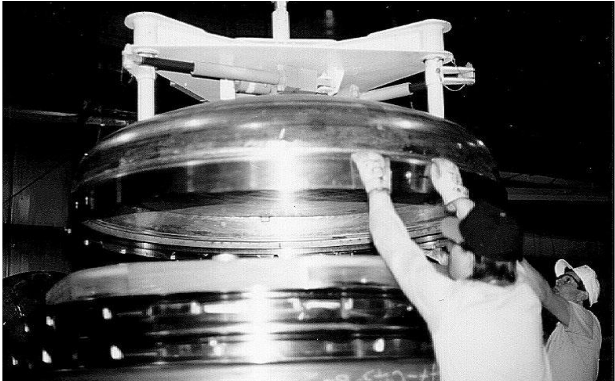
Figure 2.10.3-53 – CTU; Final ICV Lid Alignment During ICV Lid Installation
