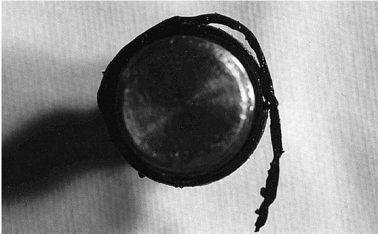
Figure 2.10.3-47 – ETU; View of OCV Vent Port Plug (As Removed; Not Cleaned)
