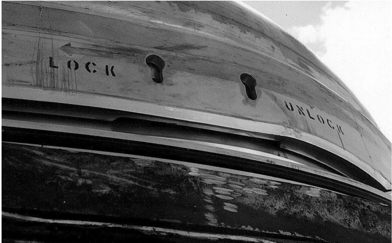
Figure 2.10.3-88 – CTU; Close-up of Damage to ICV Locking Ring
