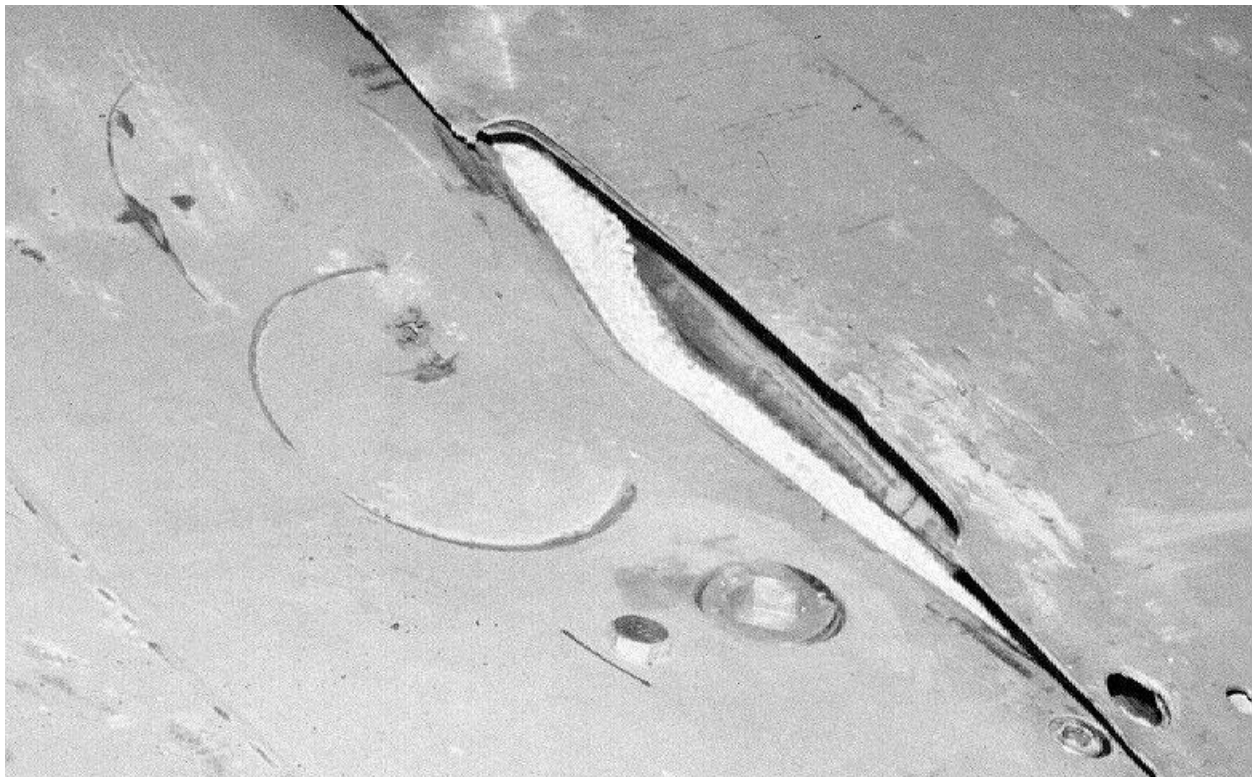
Figure 2.10.3-27 – ETU Puncture Drop Test 8; Close-up View of Damage; ~2½" Deep Dent
