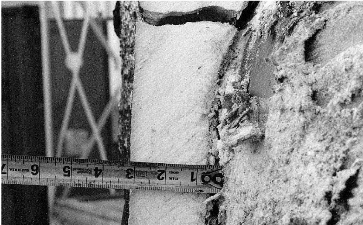
Figure 2.10.3-80 – CTU; Residual Foam in OCA Lid Side; Aligned with Test 1, 2, & 4 Damage
