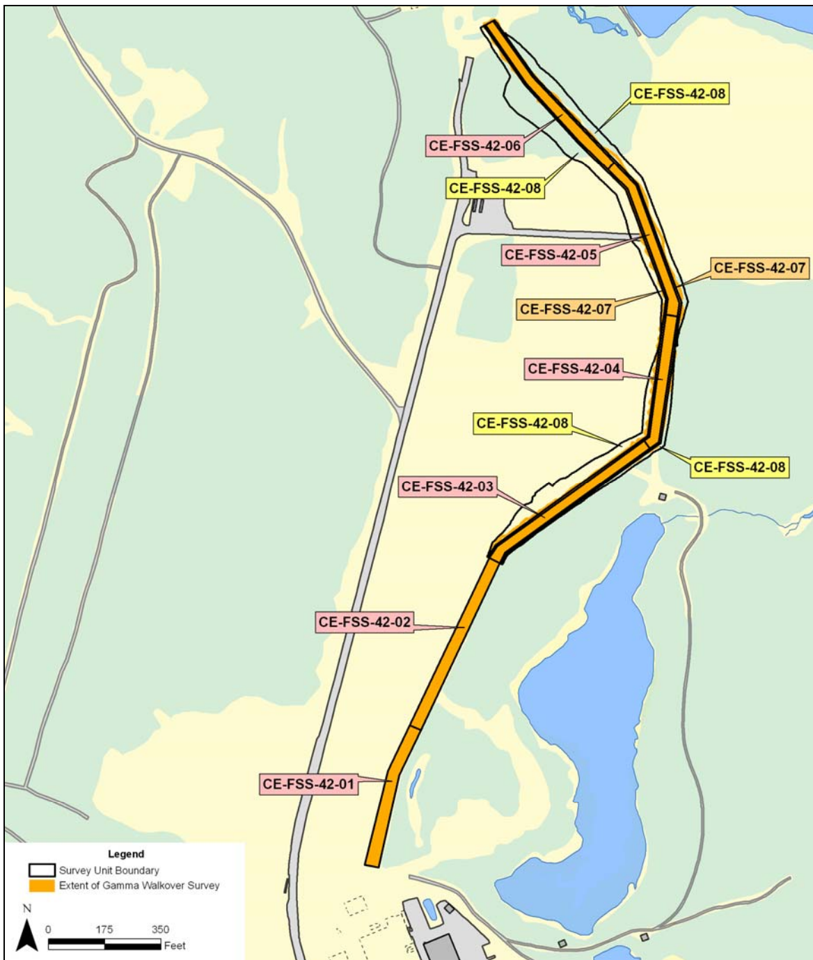
Figure 3.17: Industrial Waste Line Gamma Walkover Surveys
