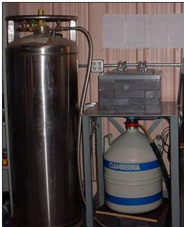
Figure 2.4: On-Site HPGe 25% Detector Shield and LN 2 Dewar
