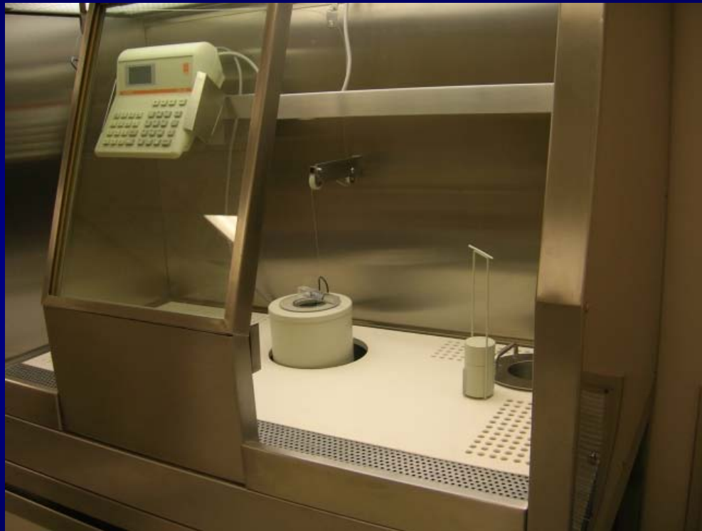
Dispensing station with dose calibrator
