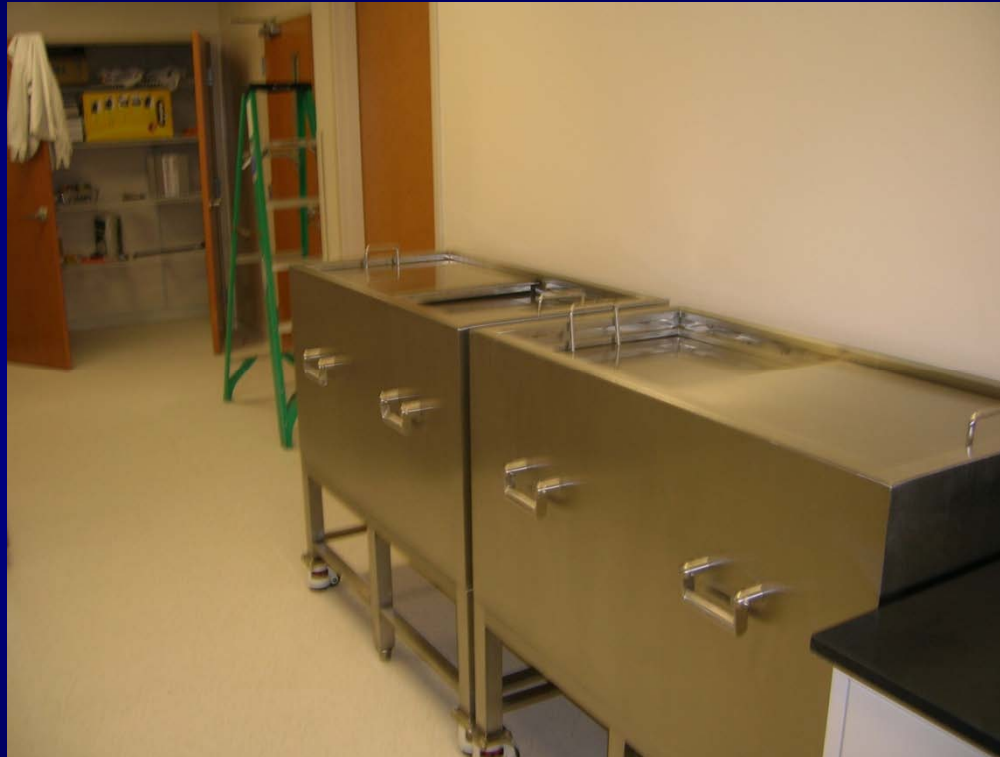
Shielded boxes for generators
