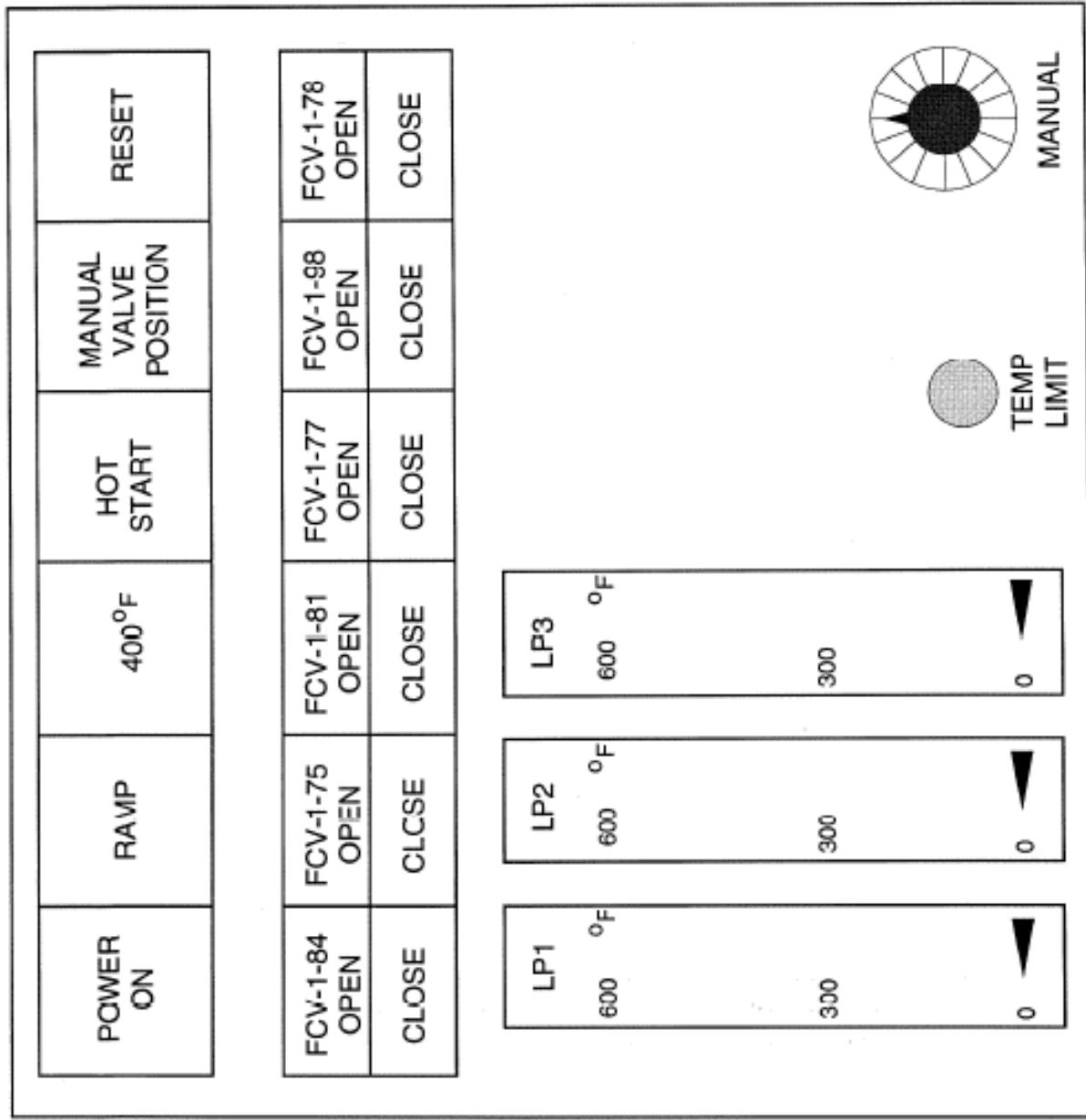
Figure 11.4-1 Reheater Control Panel
