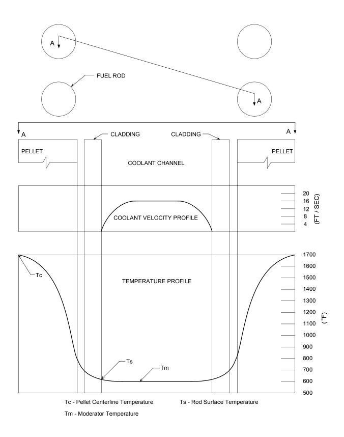
Figure 2.2-1 Local Radial Temperature and Velocity
