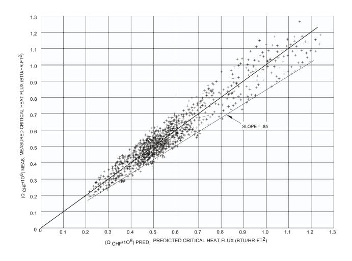
Figure 2.2-3 Measured Versus Predicted Critical Heat Flux
