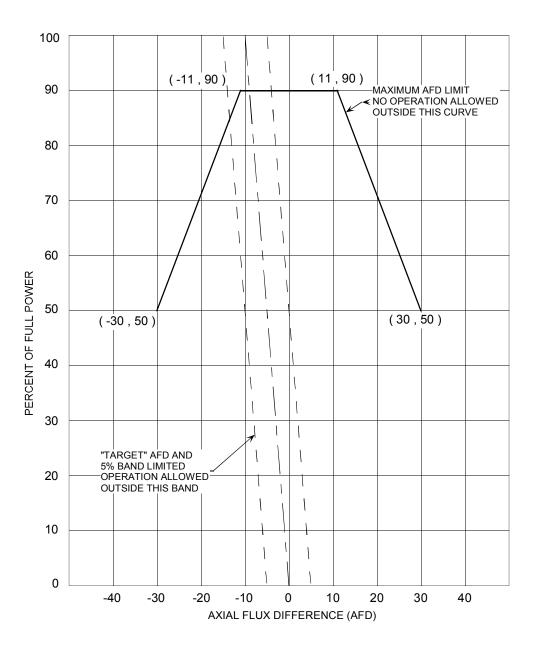
Figure 2.2-5 Axial Flux Difference Limits
