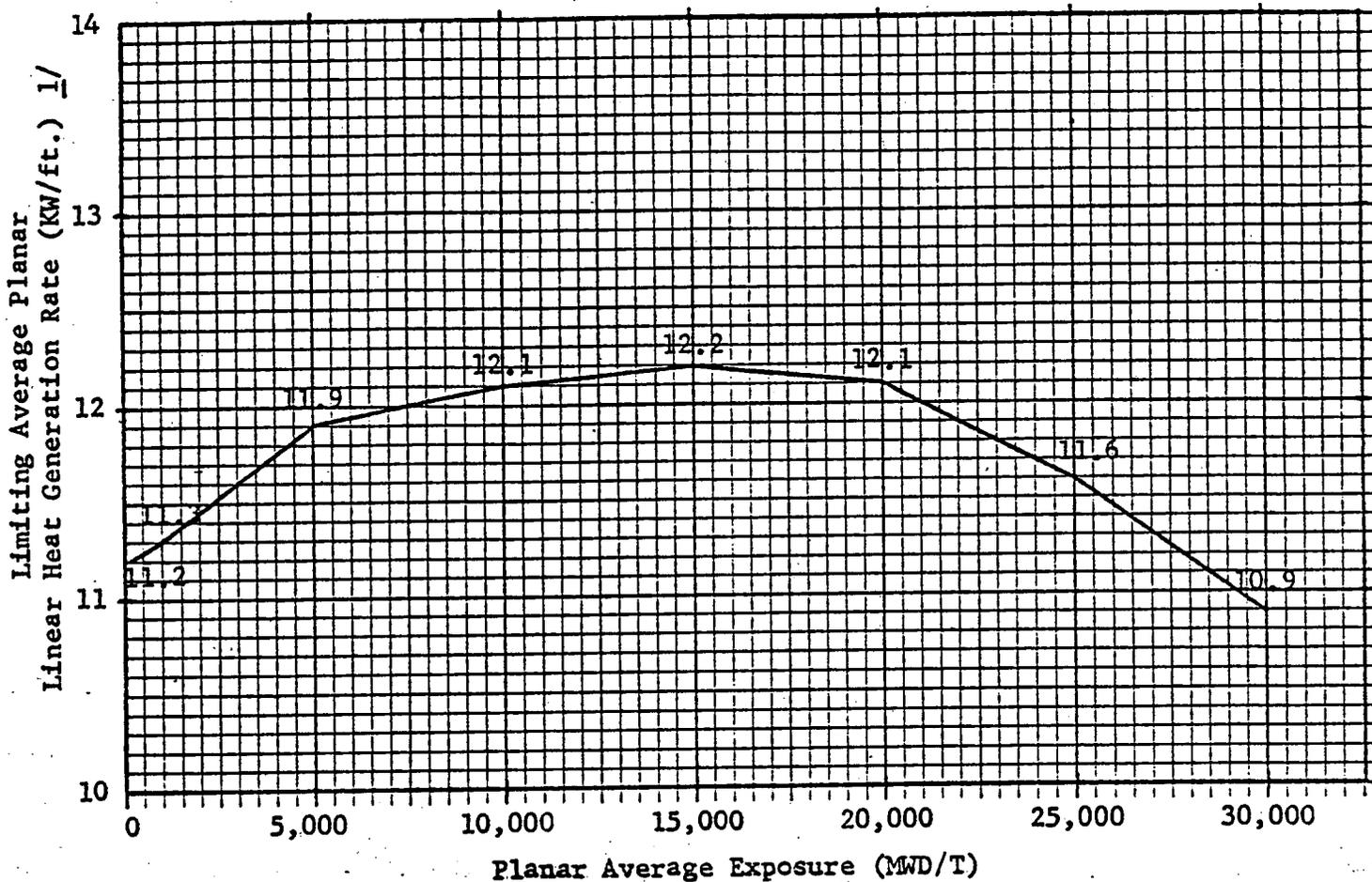
1/ When core flow is equal to or less than 70% of rated, the MAPLHGR shall not exceed 95% of the limiting values shown. Values shown are for two recirculation loops. Reduction factors for one recirculation loop operation are given in Section 3.12.A.
