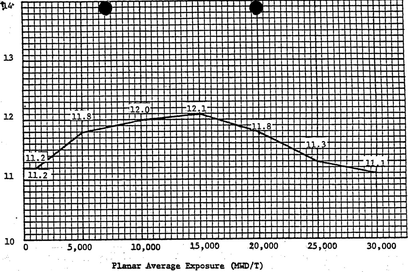
1/ When core flow is equal to or less than 70% of rated, the MAPLHGR shall not exceed 95% of the limiting values shown. Values shown are for two recirculation loops. Reduction factors for one recirculation loop operation are given in Section 3.12.A.
