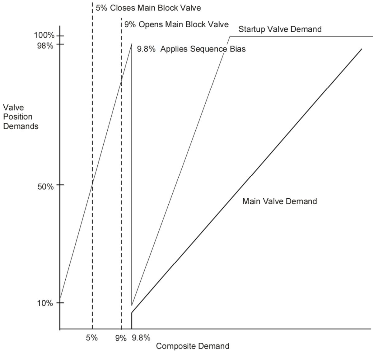
**Figure 21-3 Feedwater Valve Operations**
