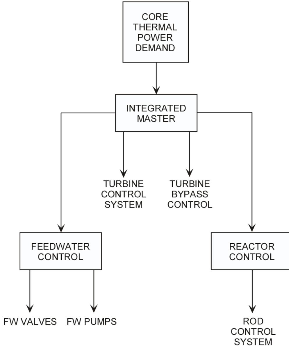
Figure 21-1 ACS Block Diagram
