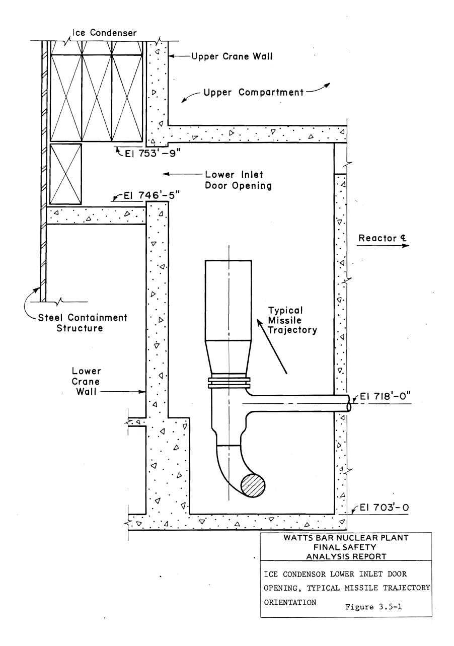
Figure 3.5-1 Ice Condenser Lower Inlet Door Opening, Typical Missile Trajectory Orientation
