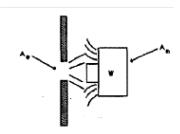
Assuming that fluid impinging on missile imparts all of its axial momentum to the missile and splashes radially out of the stream, the force balance on the missile is:
