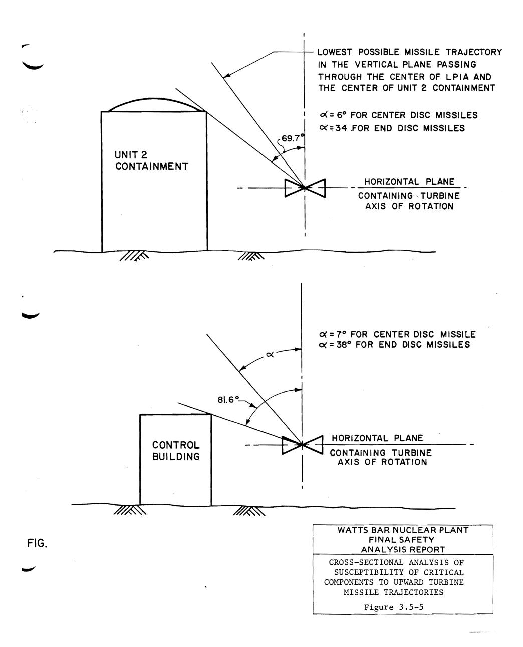
Figure 3.5-5 Cross-Sectional Analysis of Susceptibility of Critical Components to Upward Turbine Missile Trajectories
