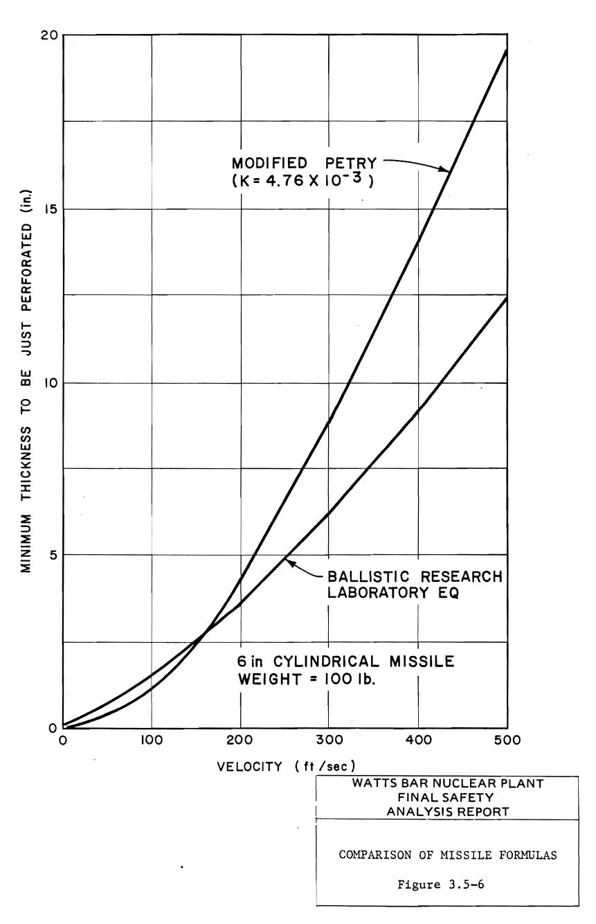
Figure 3.5-6 Comparison of Missile Formulas (6-in Cylindrical Missile)
