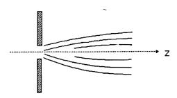
For steady flow, assuming bulk properties across a cross section of a "free jet," the following conservation relations hold between the orifice and any downstream position.
