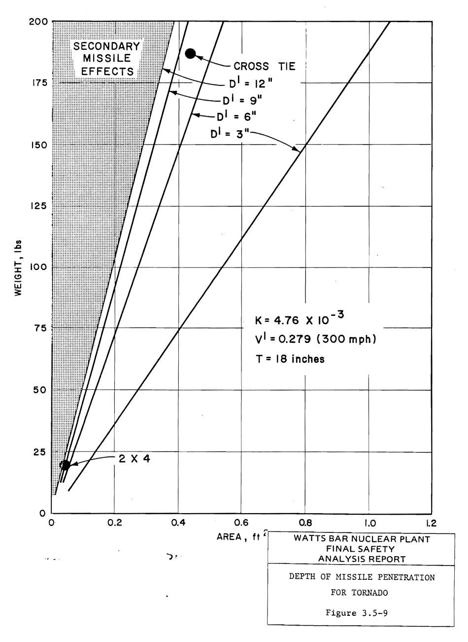
Figure 3.5-9 Depth of Missile Penetration for Tornado (2X4)
