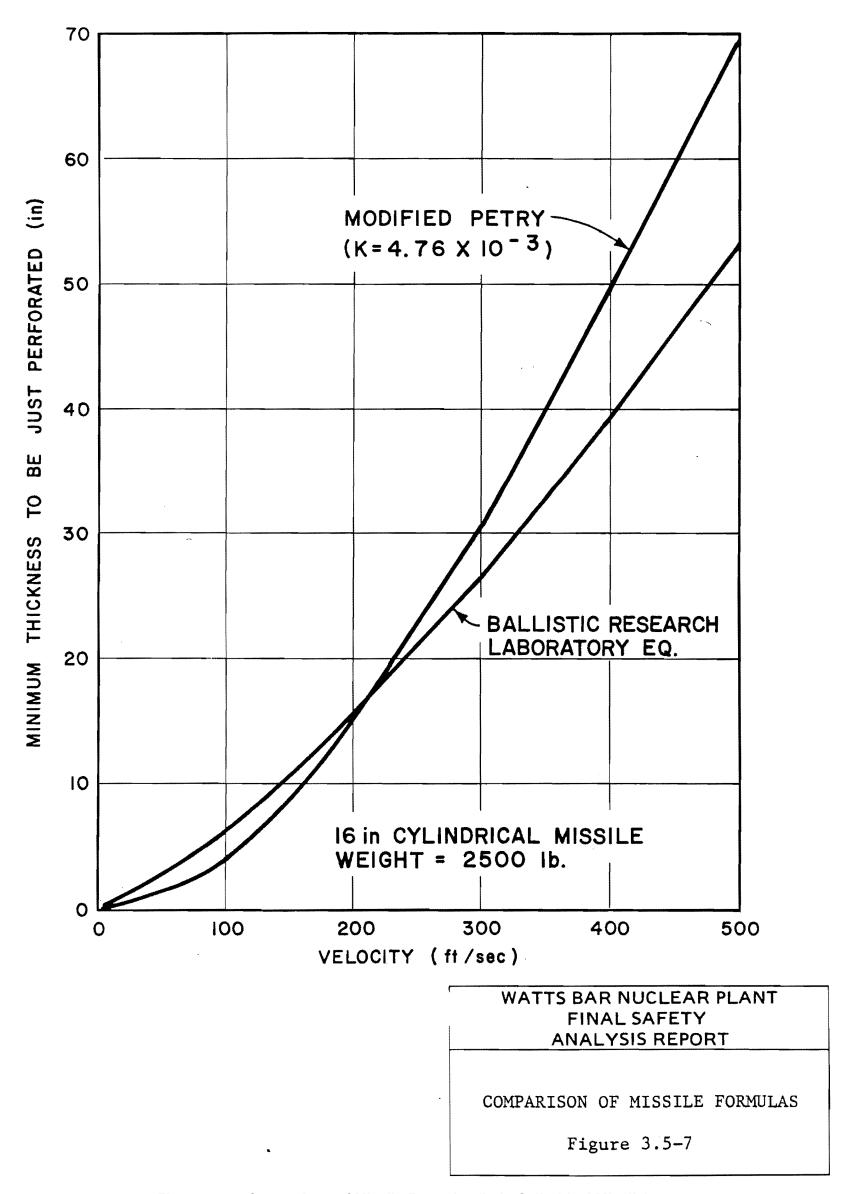
Figure 3.5-7 Comparison of Missile Formulas (I6-in Cylindrical Missile)
