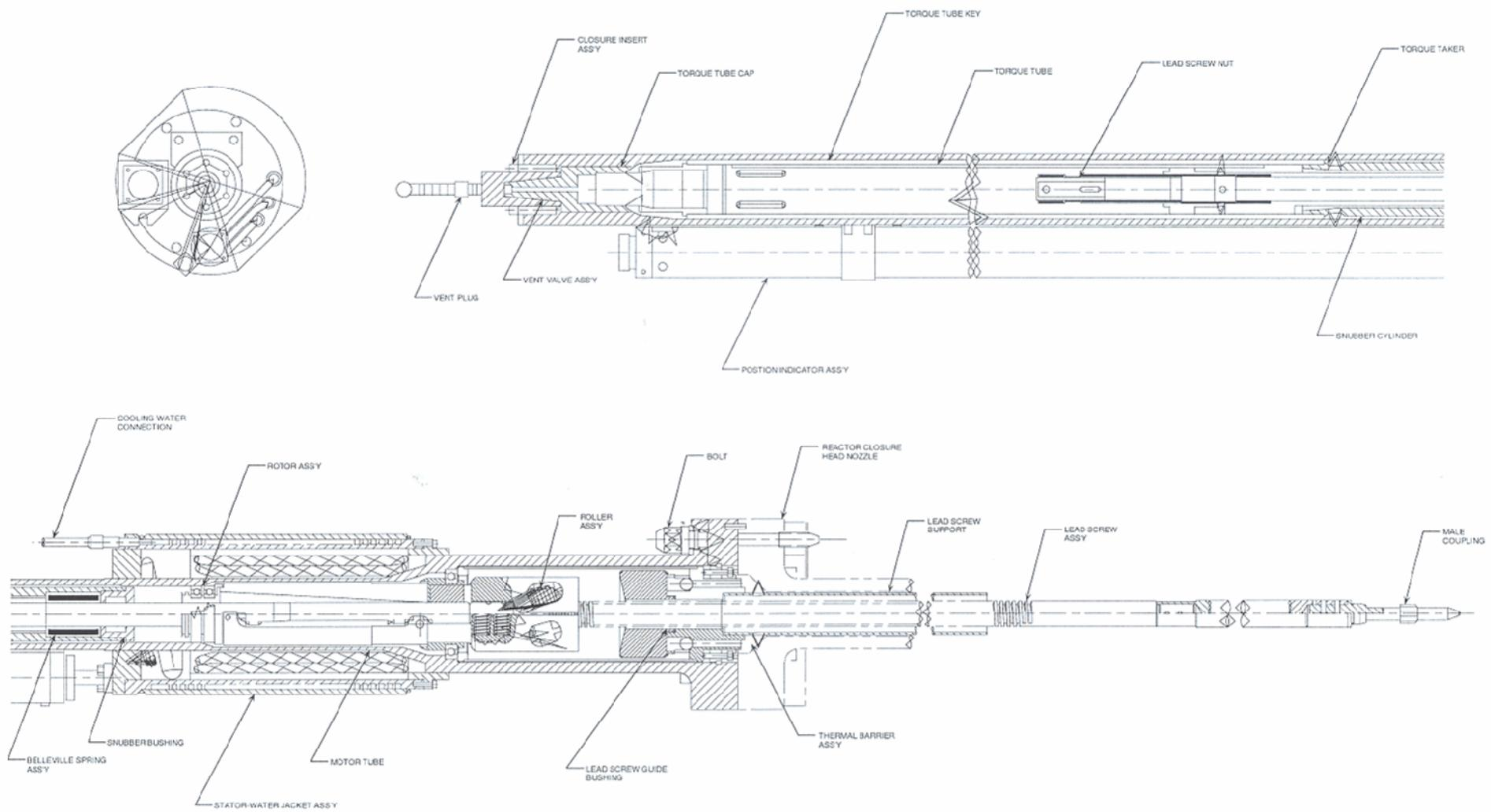
Control Rod Drive Mechanism (Fig. 6.1-2)
