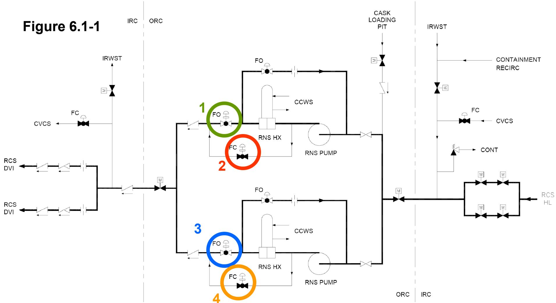
To perform cooldown and control temperature operator adjusts the positions of valves 1, 2, 3, & 4.
