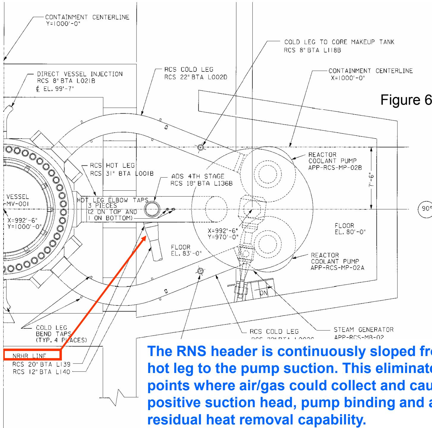
**The RNS header is continuously sloped from the RCS hot leg to the pump suction. This eliminates local high points where air/gas could collect and cause low net positive suction head, pump binding and a loss of residual heat removal capability.**
