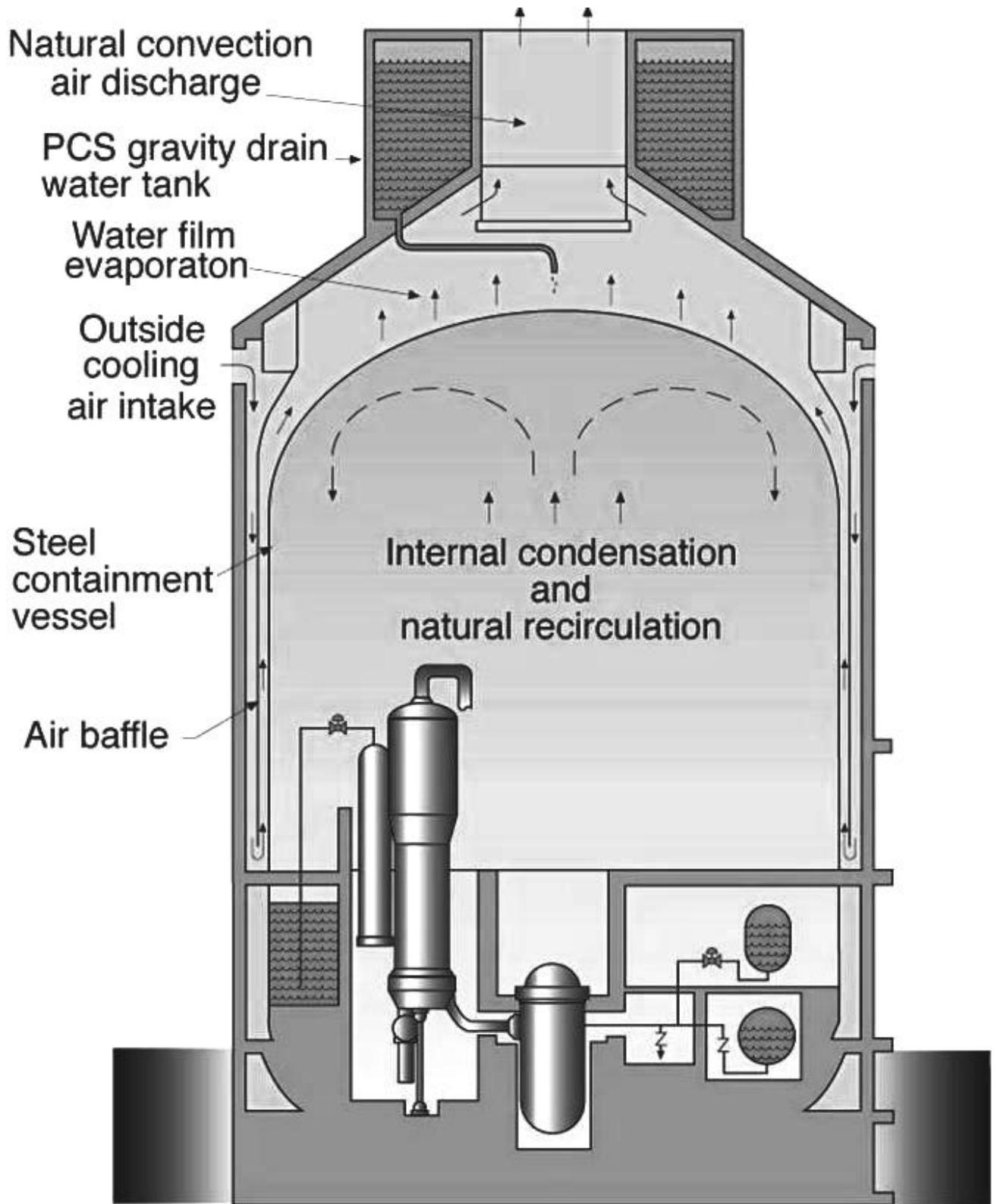
Figure 5.2-2 Containment and Shield Buildings with Passive Cooling Effects
