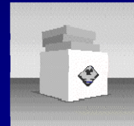
Compression test of at least 4 times the weight of the package for at least 24 hours.
