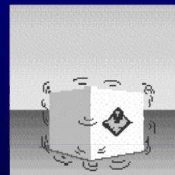
Vibration test for 4 hours on a platform vibrating so that the package will be raised high enough for a 100 m/sec (200 ft/sec) drop to be possible from the bottom of the package and the platform.
