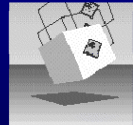
Free drop test into a test, hard surface (7.6 m/sec (24.6 ft/sec) drop if the package weighs 4,500 g (10 lb) or less.
