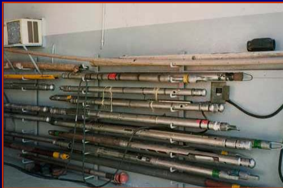
Well Logging tools (without sources) at storage facility
