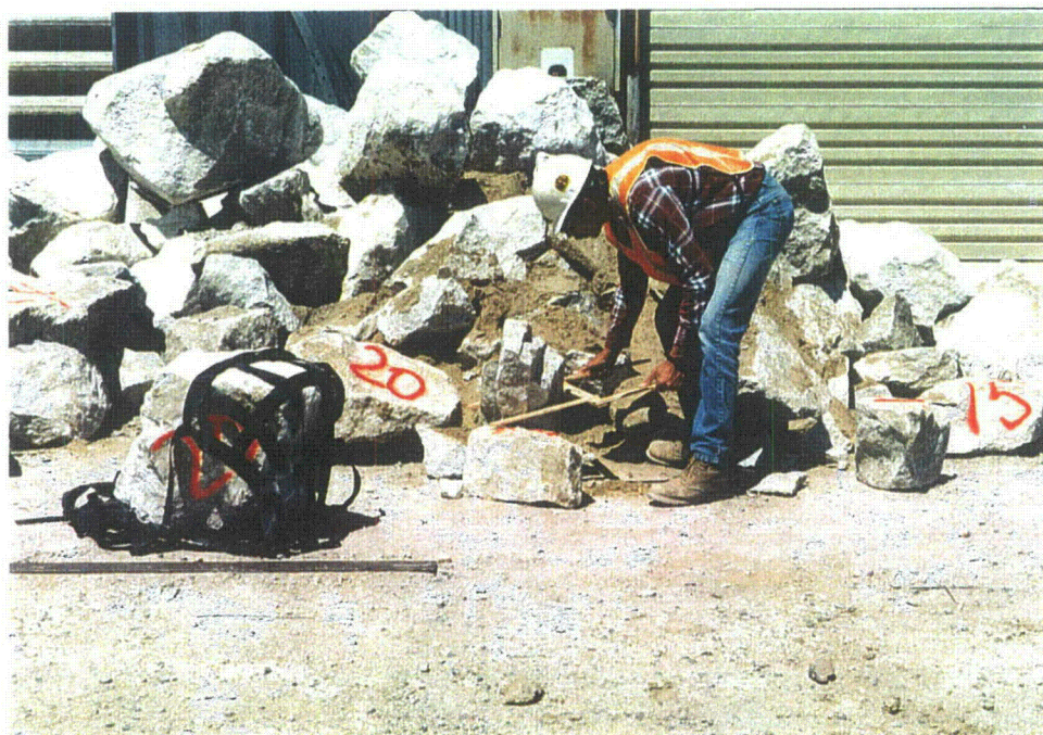
Photo 32 – Gradation testing D 50 18" riprap, September, 1995
