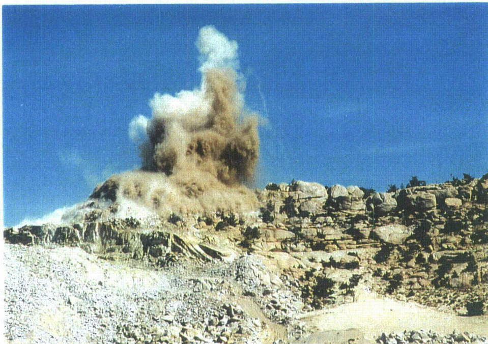
Photo 31 - Blasting at rock quarry to make granite erosion control mulch and riprap, September, 1995
