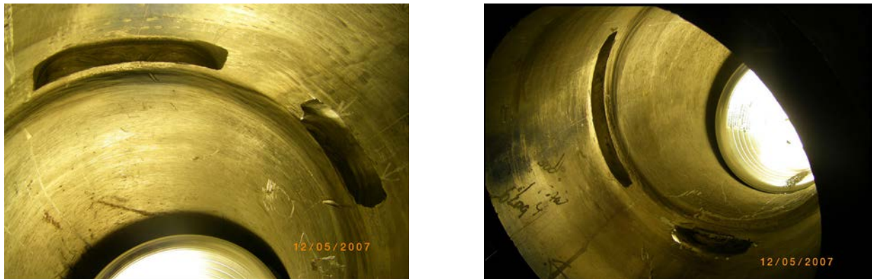
Figure 7.1. Photographs of the Inside Surface of the CASS PZR Surge-Line After Excavation and Preparation of the Areas Targeted for Flaw Implantation (courtesy of FlawTech ® , Inc.)
