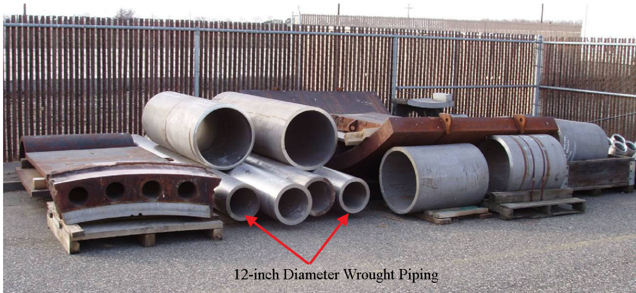
Figure 7.3. Photographs of the WSS Parent Material from which the Two Calibration Coupons (with EDM notches) were Extracted
