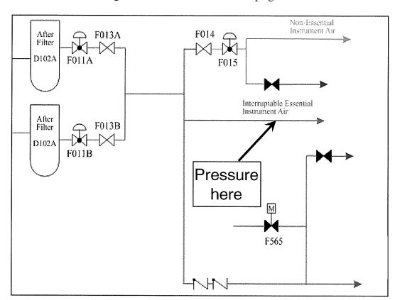
If NO operator action is taken, which ONE of the following choices correctly states how the plant will respond to this instrument air pressure reduction?
