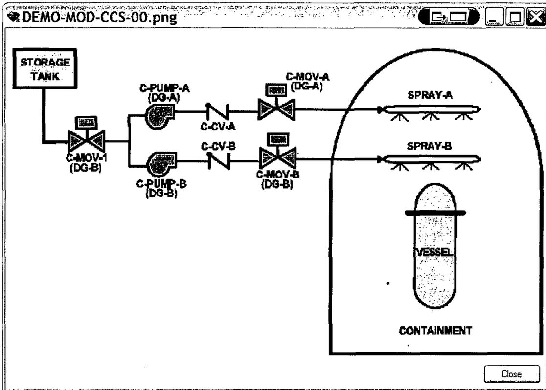
Figure 17. Example P&ID for the CCS system
