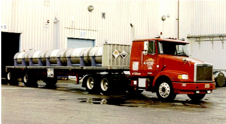
Figure 2-7 Truck Loaded with Five 30B Enriched Product Cylinders Loaded for Transport in Their Protective Overpacks (DOE, undated b)
