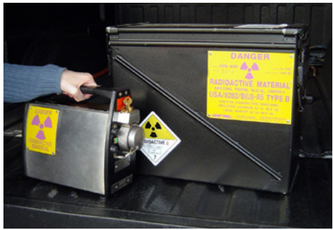
A radiography camera and its approved transport container.
