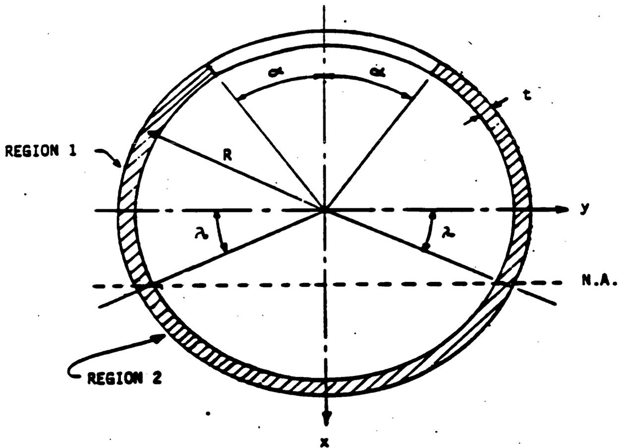
Figure A-1. Cross Section Of Pipe With A Through-Wall Circumferential Crack of Length  $2\alpha$ .
