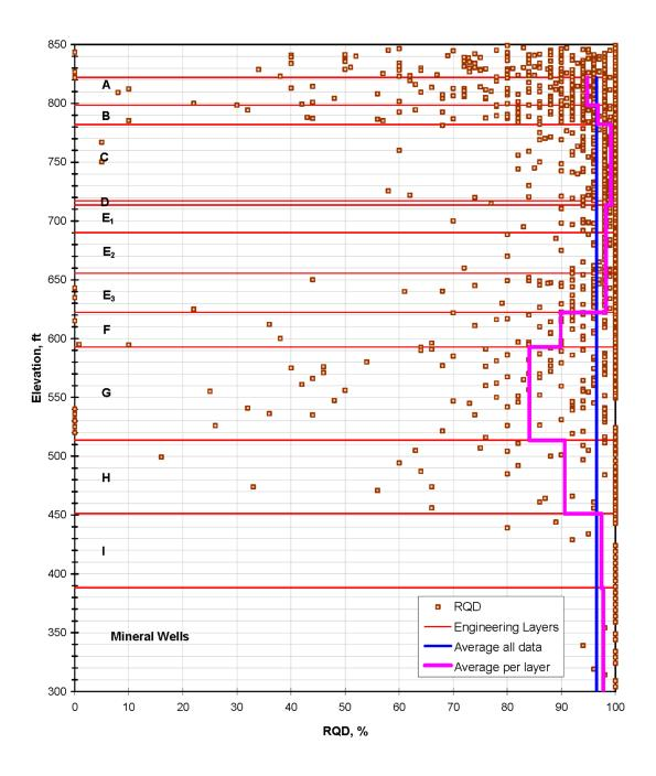
Figure 2.5.4-240 Rock Quality Designation vs. Elevation
