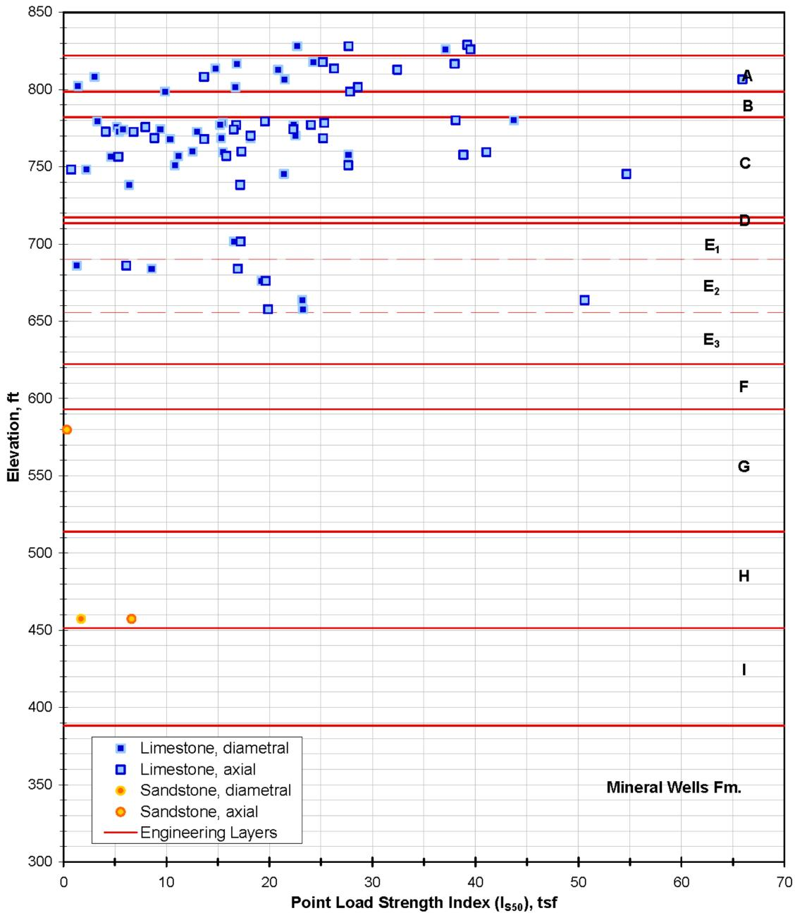
**Figure 2.5.4-228 Point Load Strength Index vs. Elevation**
