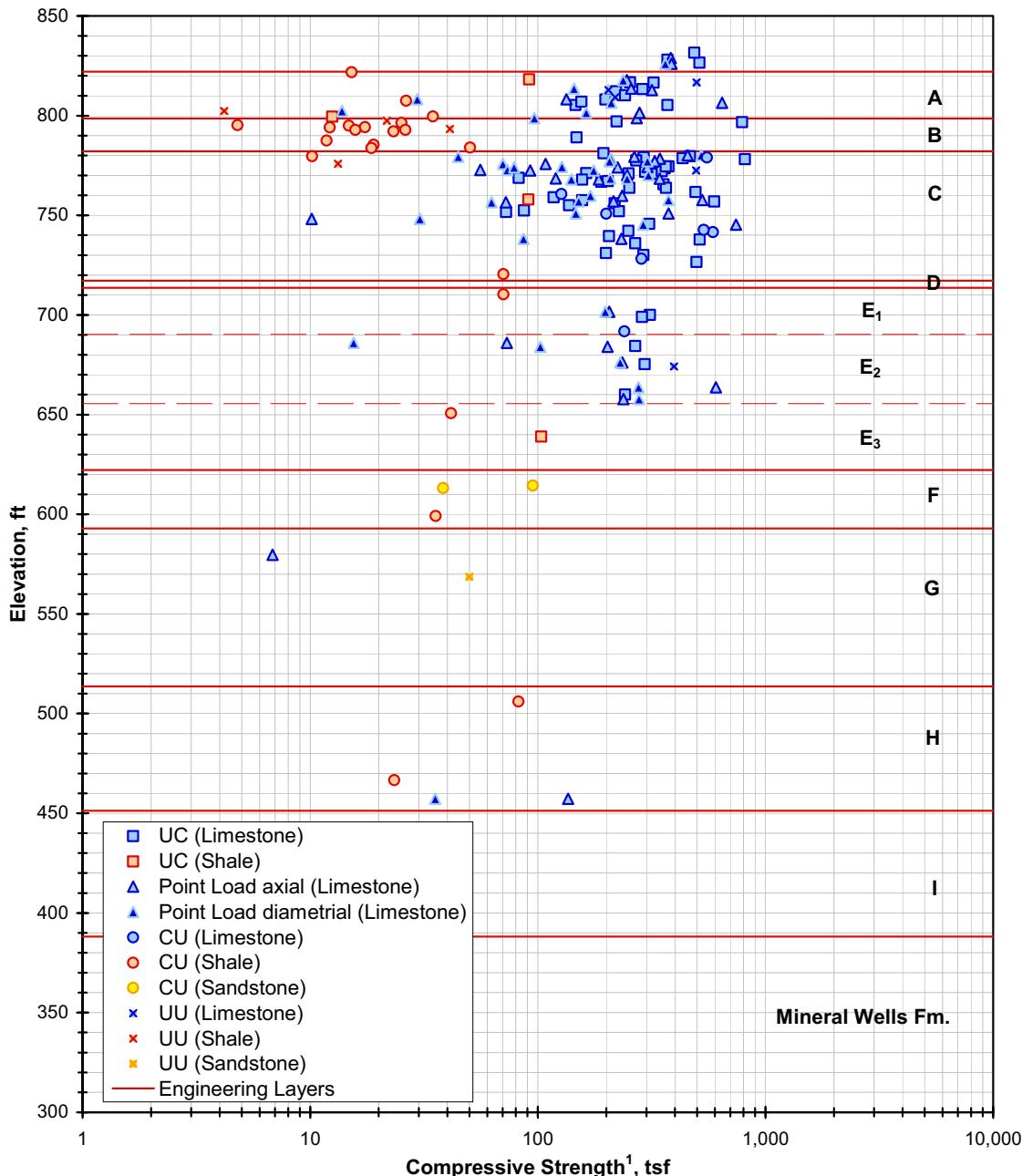
**Figure 2.5.4-227 Compressive Strength vs. Elevation**
