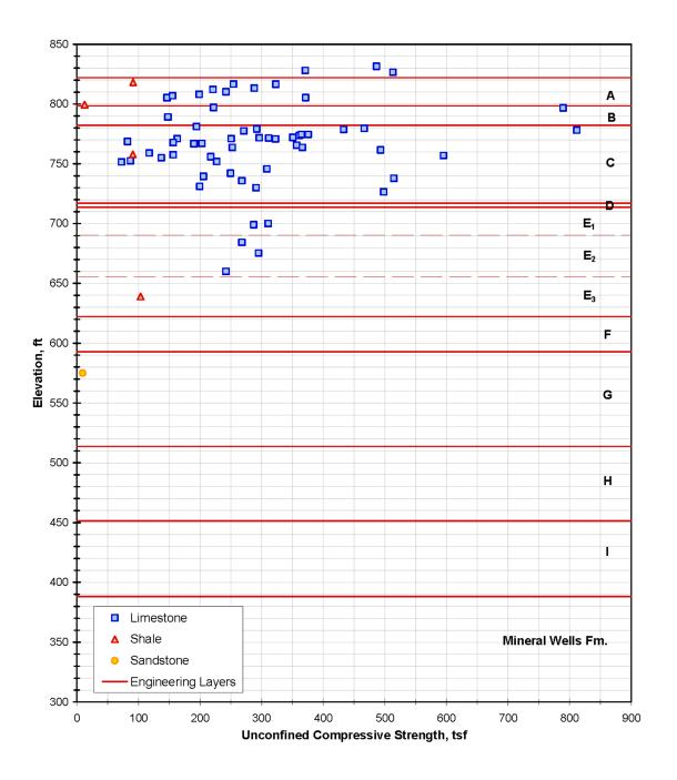
Figure 2.5.4-226 Unconfined Compressive Strength vs. Elevation
