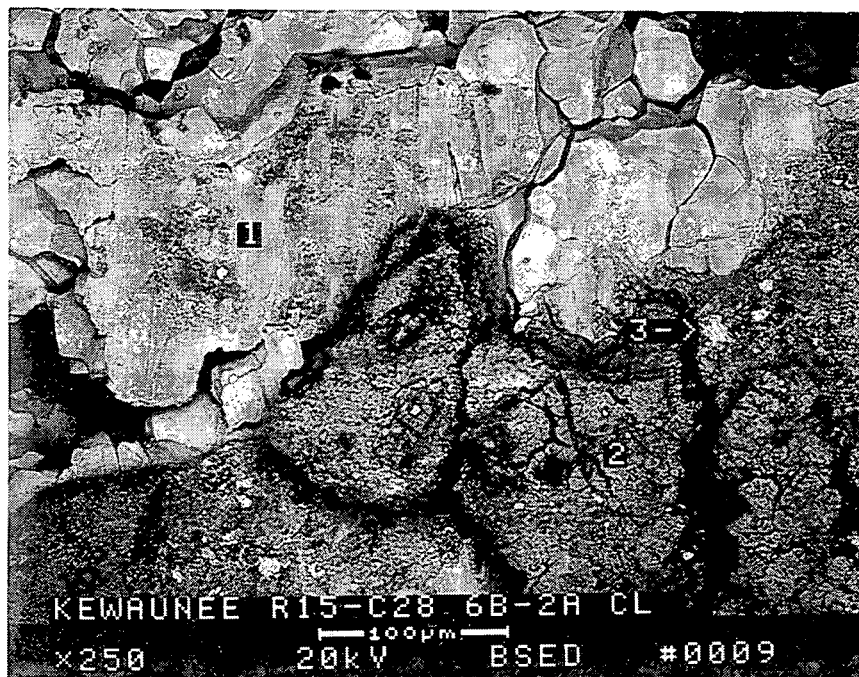
Figure 4-41 TSP2 crevice region Specimen 6B-2A of Tube R15C28. Side view of the opened burst fracture showing OD corrosion cracks opened wider by the burst test. Higher magnification photographs of Areas 7 and 9 on the OD surface from Figure 4-37, showing the locations of Spots 1, 2, and 3 which were analyzed using the energy dispersive X-ray spectroscopy (EDS) technique. The results of the analyses are shown in Figures 4-42, 4-43, and 4-44.
