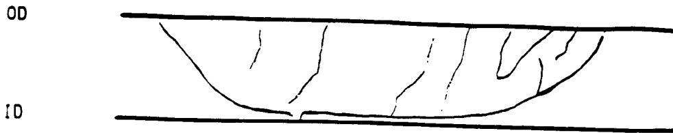
Sketch of Burst Crack
