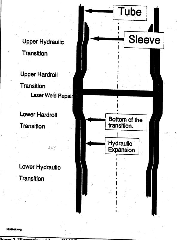
Figure 2. Illustration of Laser Weld Repair in Kewaunee HEJ Upper Joint
