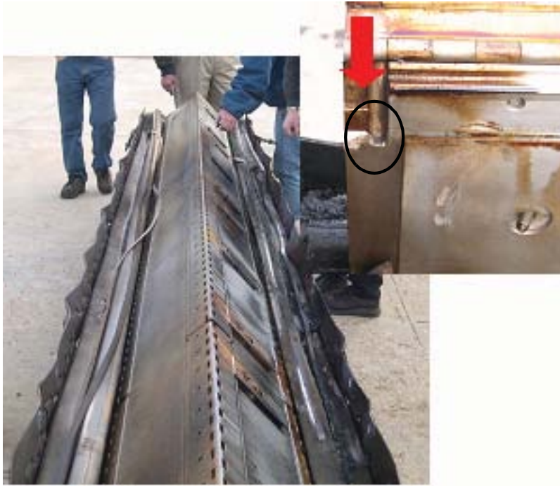
Figure 2-149 CTU Clamshell After Drop and Fire Tests
