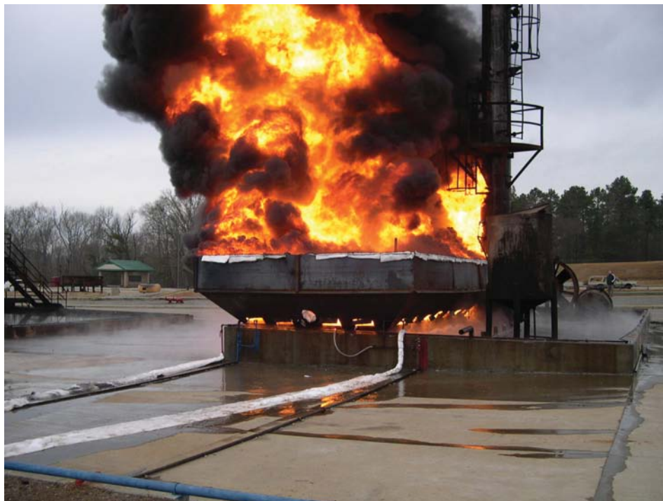
Figure 3-4 December 15, Impact Limiter Burn Test
