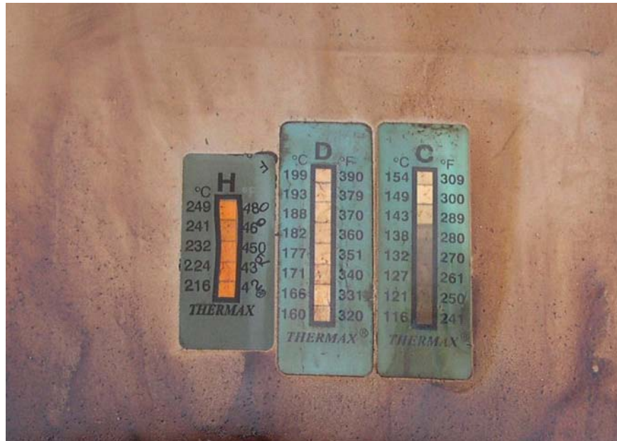
Figure 3-8 Temperature Strip Condition After CTU Burn Test
