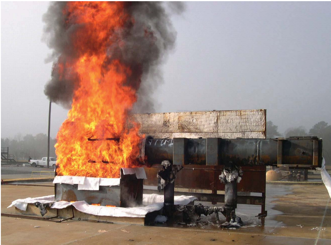
Figure 3-19 December 15, Impact Limiter Burn Test
