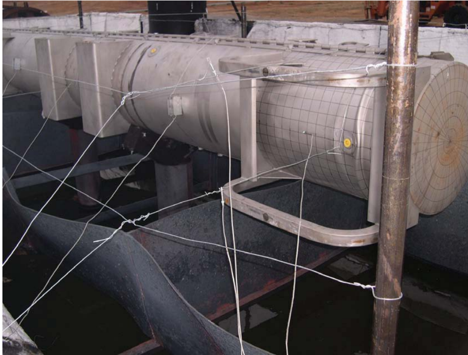
Figure 3-32 Test Stand for Fire Test
