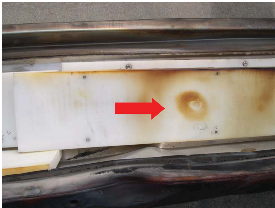
Figure 3-44 Localized Melt Spot in Lid Moderator Block
