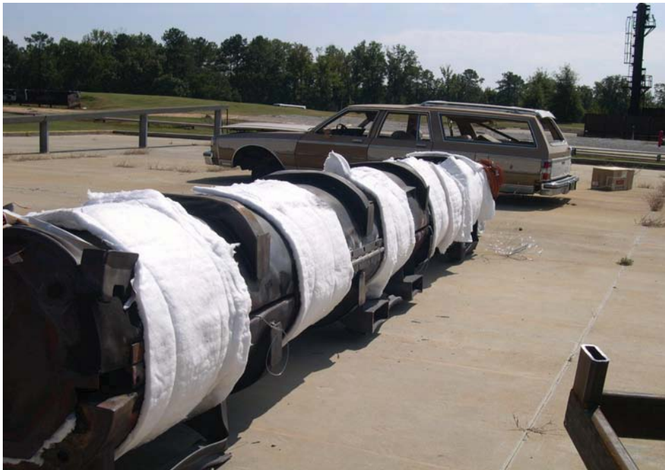
Figure 3-11 Package Exterior Wrapped with Ceramic Fiber Insulation
