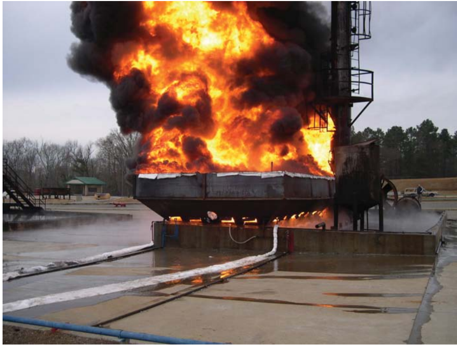
Figure 3-6 Traveller CTU During Pool Fire Test
