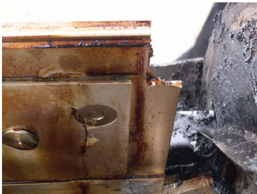
Figure 3-31 Brown Polyurethane Residue Inside Outerpack After Burn Test
