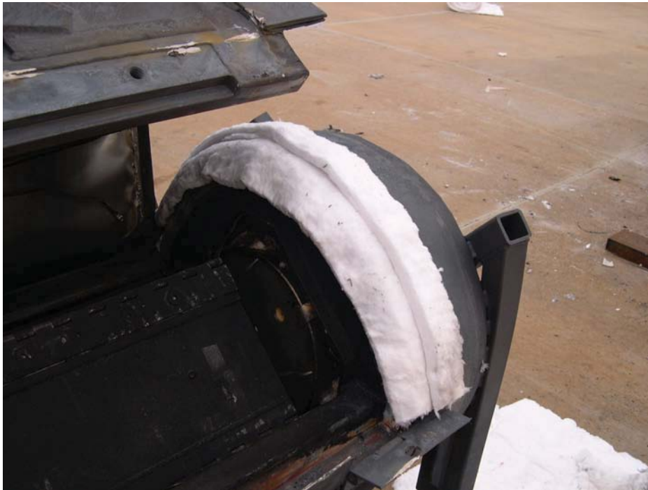
Figure 3-24 Kaowool Layers on Outerpack Bottom Impact Limiter
