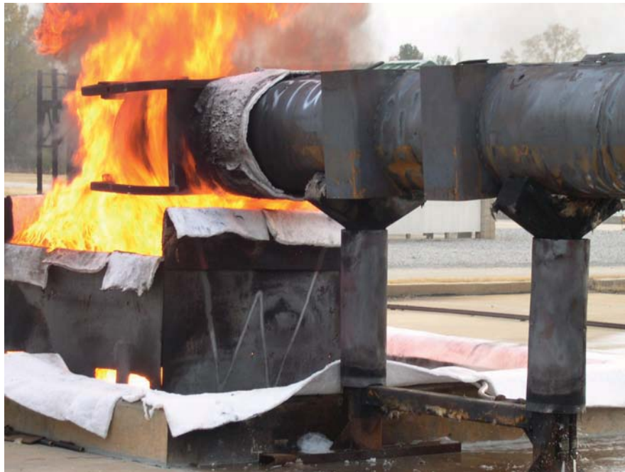
Figure 3-25 December 16 Impact Limiter Burn
