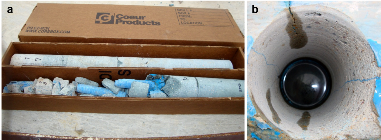
Figure 3-5. (a) Photograph of Overcores 7 and 8 Illustrates the Rubblized Zone of Grout and Blue Epoxy that Comprise the Top of Overcore 8. (b) View Into Corehole 8 Supports Staff Recommendation To Conduct Future Borescopic Observations in Coreholes 1–9.
