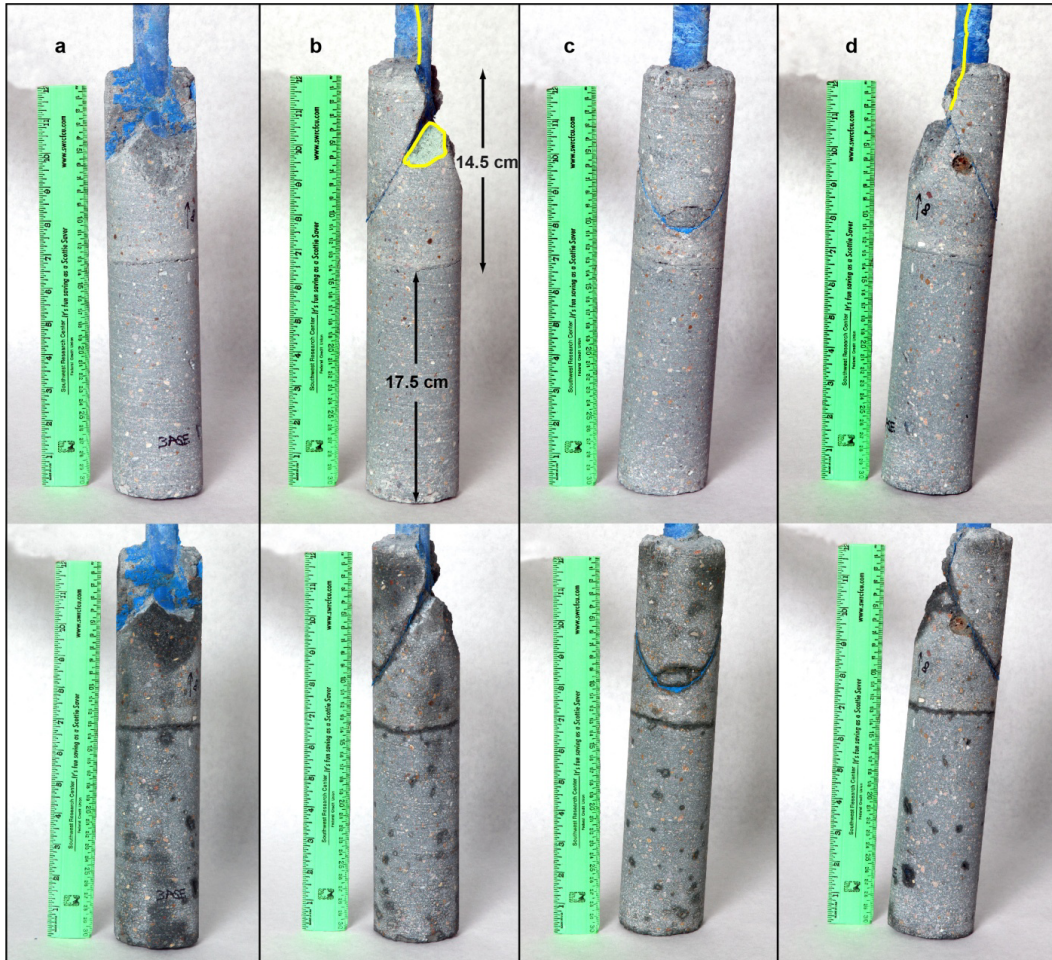
Figure 3-6. Intact Section From Overcore 8 From Base to Height of 32 cm [12.6 in] Shown Dry (Top) and Wet (Bottom). Core Was Turned Counterclockwise in ~90° Increments for Each Photograph.
