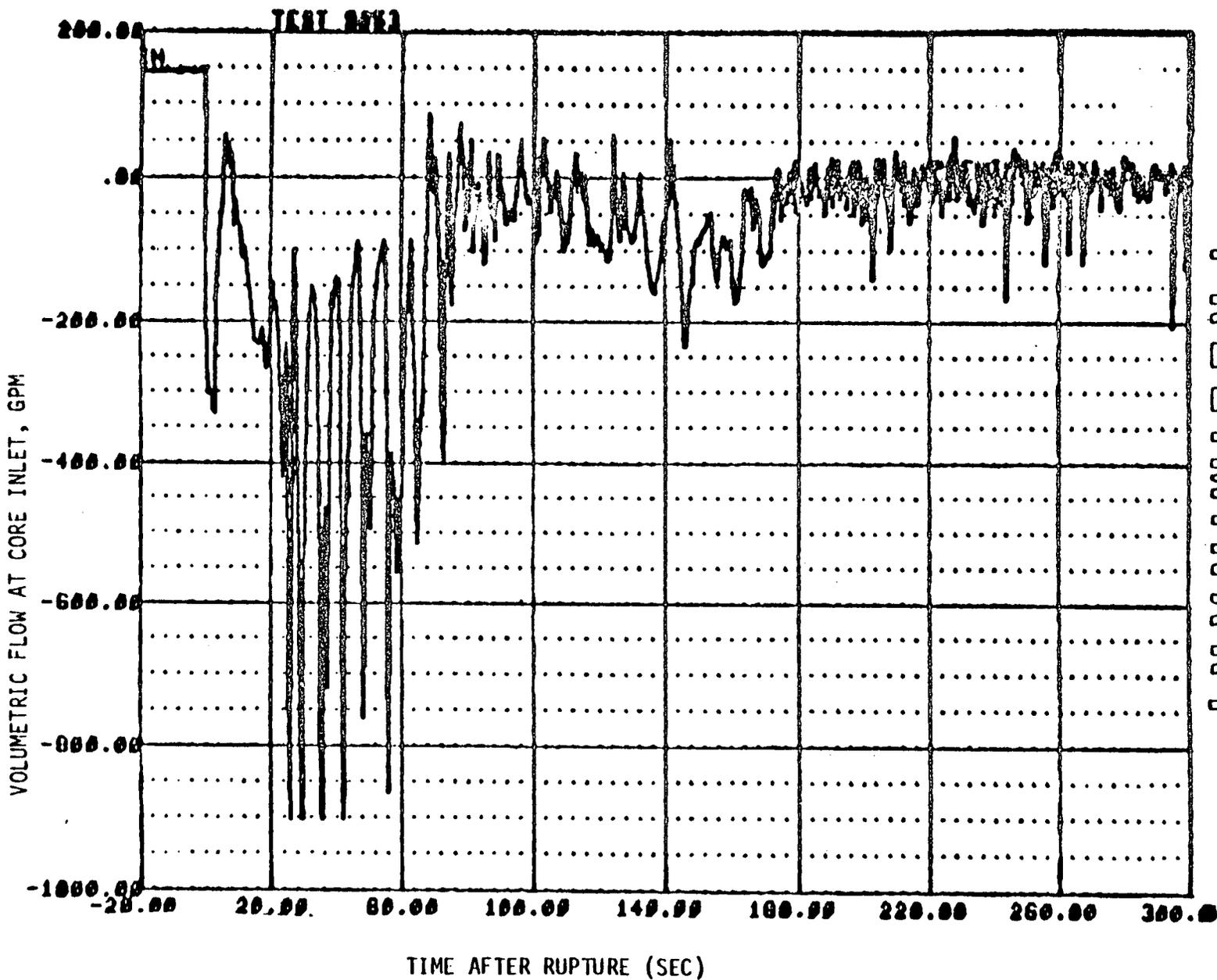
Volumetric Flow Rate at Core Inlet (Test S-05-3)
