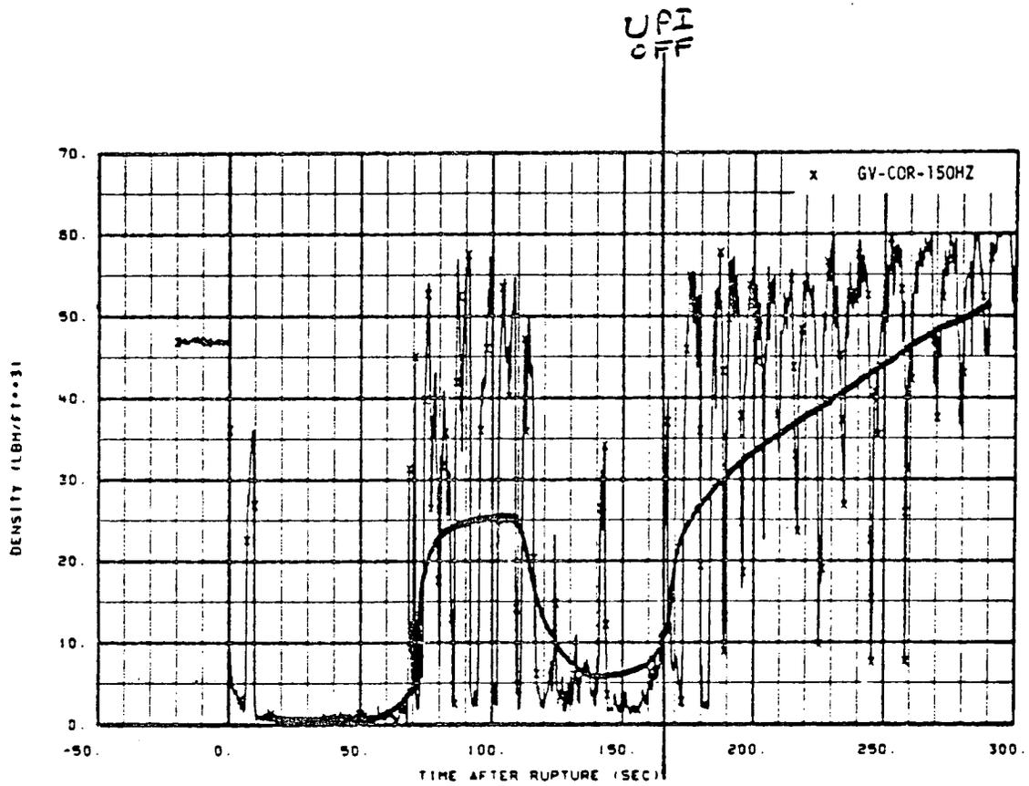
Fig. 283 Density in vessel (GV-COR-150HZ), from -20 to 300 sec.
